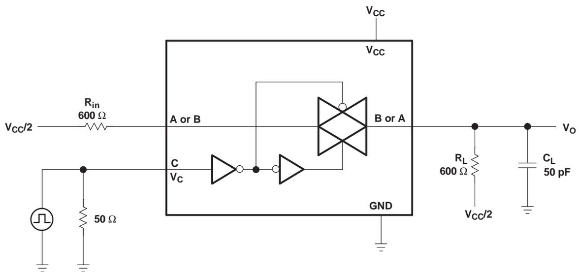
Figure 7. Crosstalk (Control Input – Switch Output)
