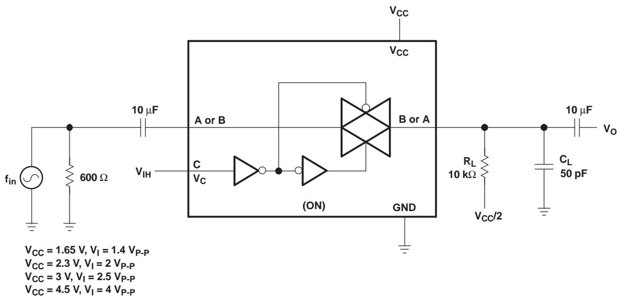
**Figure 9. Sine-Wave Distortion**
