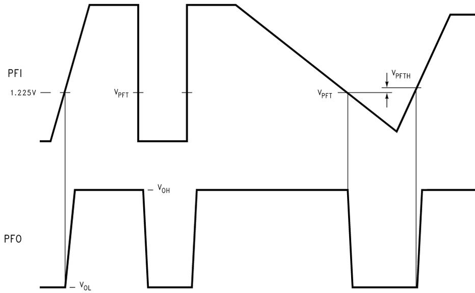
Figure 3. PFI Comparator Timing Diagram
