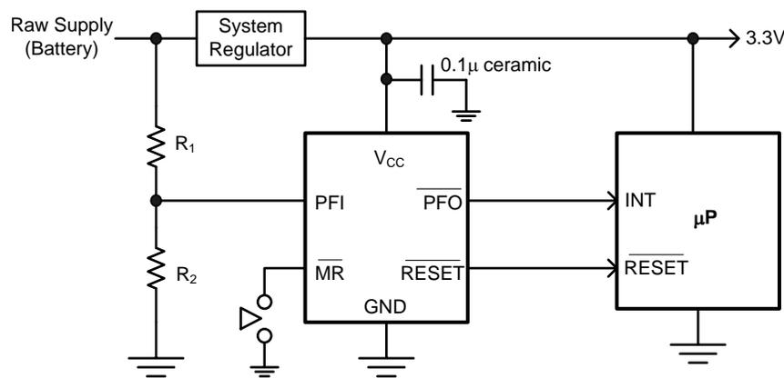
$$\text{Power-Fail Reset Threshold, } V_{PFT} = 1.225 \left( \frac{R_1}{R_2} + 1 \right)$$
