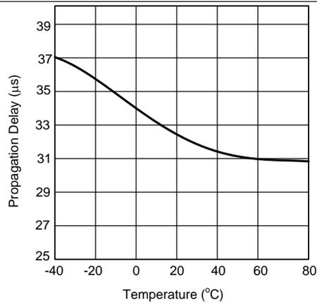
**Figure 10. Low-Line Comparator Propagation Delay vs Temperature**
