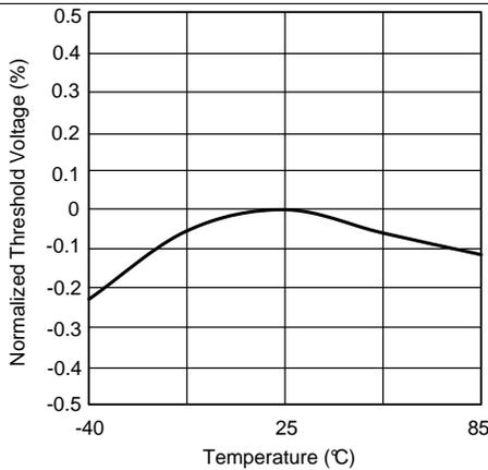
Figure 6. Normalized Reset Threshold Voltage vs Temperature
