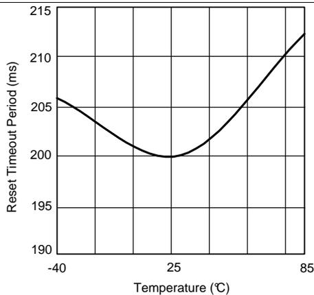
Figure 8. Reset Timeout Period vs Temperature
