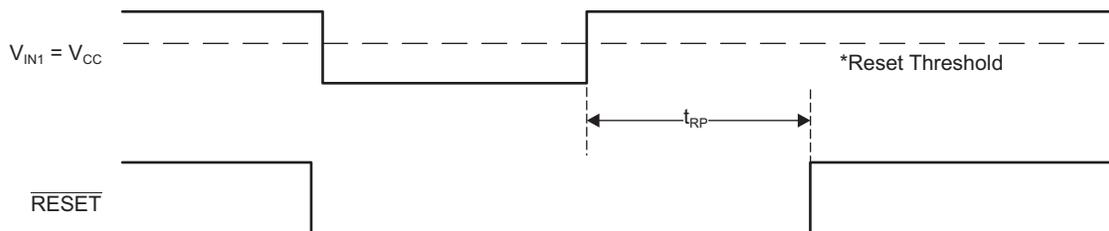
Standard reset threshold is 3.08 V. Custom reset voltages are available between 2.2 V and 5 V in 10-mV increments by contacting Texas Instruments.
