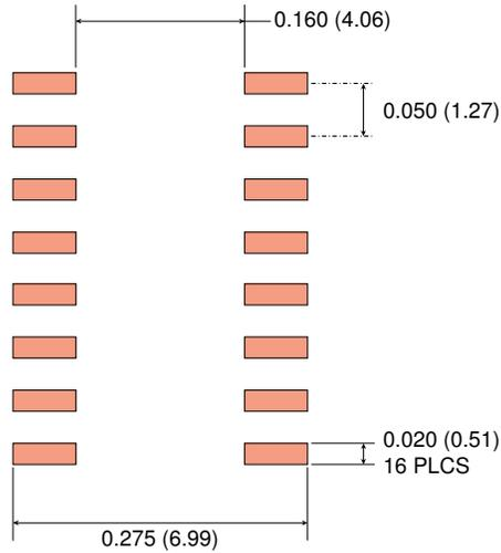
**0.3" 16-pin SOIC Pad Layout**
