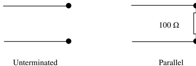
Proper termination is imperative when using IL3485 and IL3422 to minimize reflections. Unterminated lines are only suitable for very low data rates and very short cable runs, otherwise line reflections cause problems. Parallel terminations are the most popular. They allow high data rates and excellent signal quality.
