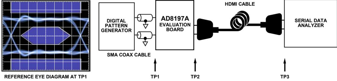
Figure 9. Test Circuit Diagram for Tx Eye Diagrams
