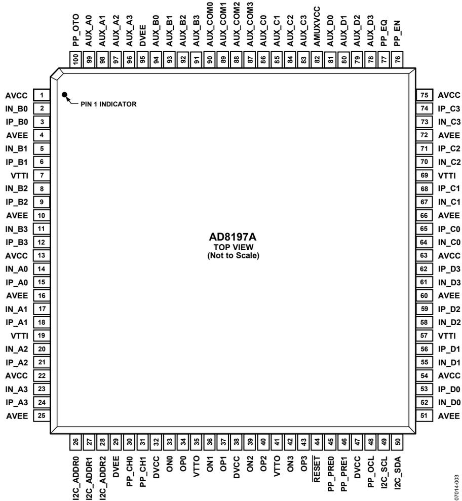
Figure 3. Pin Configuration
