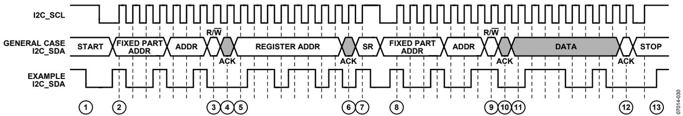
Figure 30. I<sup>2</sup>C Read Diagram
