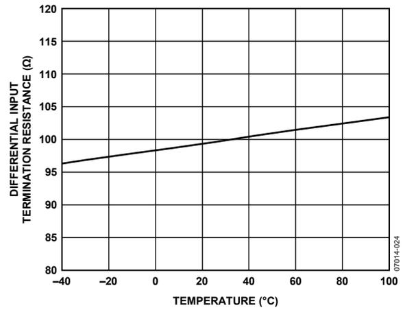
Figure 24. Differential Input Termination Resistance vs. Temperature
