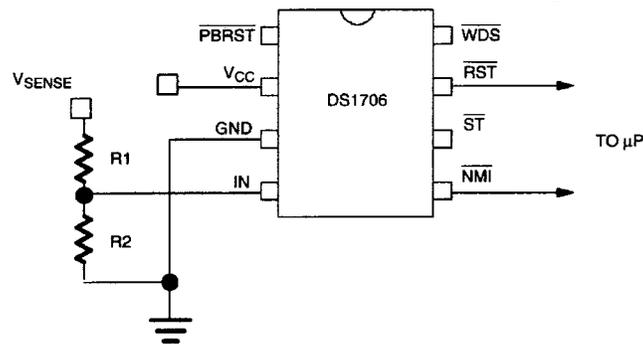
$$V_{\text{SENSE}} = \frac{R1 + R2}{R2} \times 1.25$$
