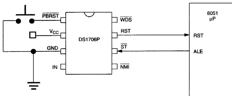
**PUSH-BUTTON RESET CONTROLLED BY  $\overline{\text{NMI}}$  AND  $\overline{\text{WDS}}$  Figure 3**
