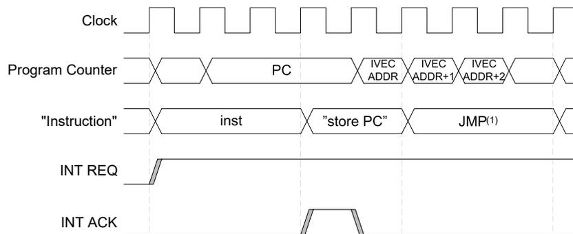
If an interrupt occurs when the device is in a sleep mode, the interrupt execution response time is increased by five clock cycles, as shown in the figure below. Also, the response time is increased by the start-up time from the selected sleep mode.
