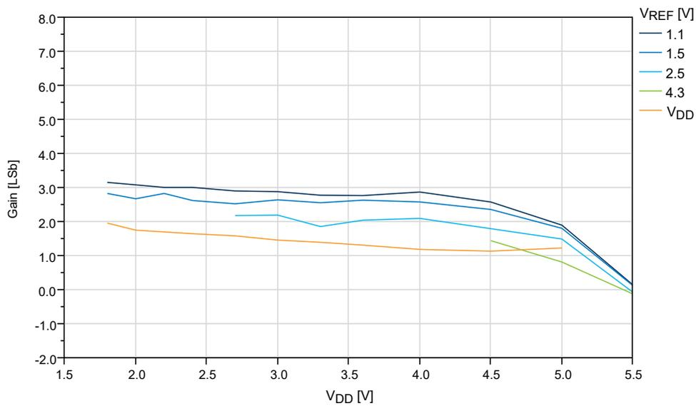
**Figure 32-45. Gain Error vs.  $V_{REF}$  ( $V_{DD} = 5.0V$ ,  $f_{ADC} = 115$  kps), REFSEL = Internal Reference**
