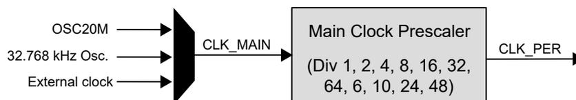
The Main Clock and Prescaler configuration (CLKCTRL.MCLKCTRLA, CLKCTRL.MCLKCTRLB) registers are protected by the Configuration Change Protection Mechanism, employing a timed write procedure for changing these registers.
