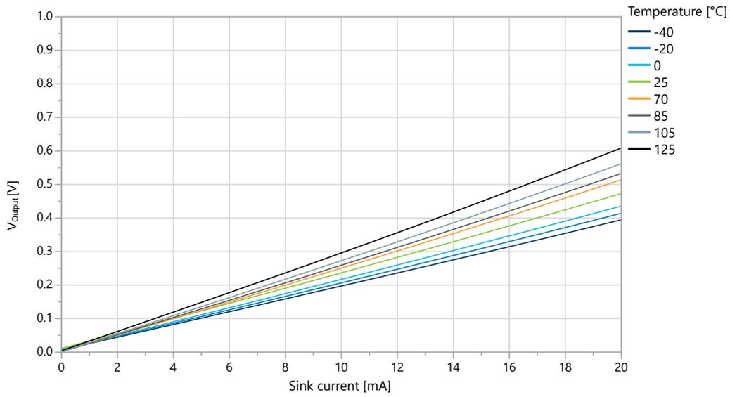
Figure 32-22. I/O Pin Output Voltage vs. Sink Current ( $T = 25^{\circ}C$ )
