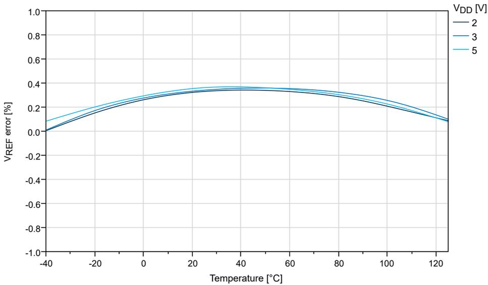
**Figure 32-31. Internal 1.1V Reference vs. Temperature**
