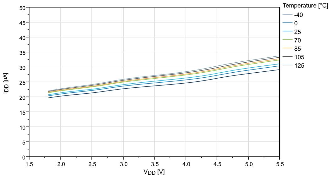
**Figure 32-35. BOD Current vs.  $V_{DD}$  (Sampled BOD at 125 Hz)**
