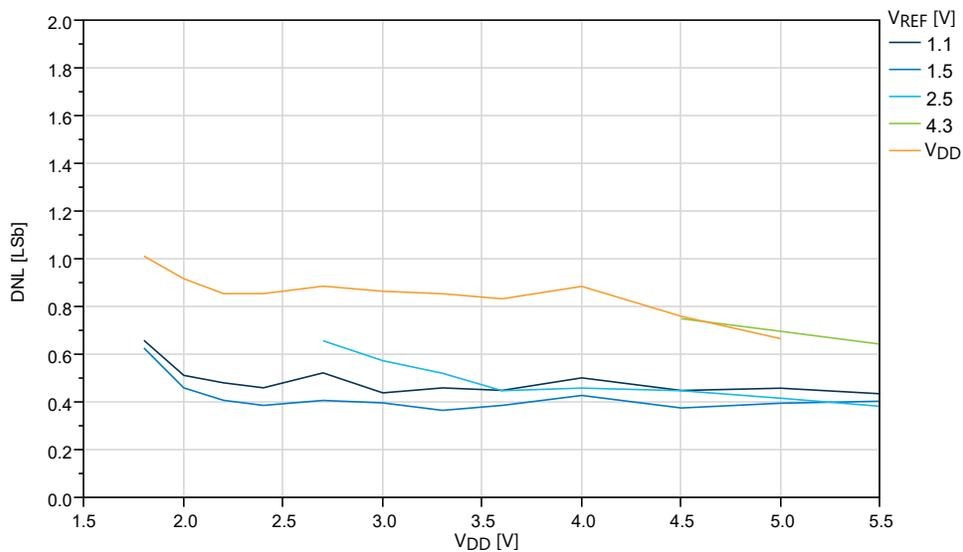
**Figure 32-43. DNL vs.  $V_{REF}$  ( $V_{DD} = 5.0V$ ,  $f_{ADC} = 115$  kps), REFSEL = Internal Reference**
