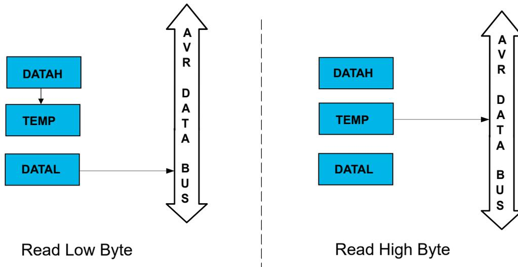
For a 16-bit read operation, the low byte register (e.g. DATAL) of the 16-bit register must be read before the high byte register (e.g. DATAH). When the low byte register is read, the high byte register of the 16-bit register is copied into the temporary (TEMP) register in the same clock cycle, as shown in the left side of Figure 8-7. Reading the high byte register will result in a read from TEMP instead of the high byte register, as shown in right side of Figure 8-7.
