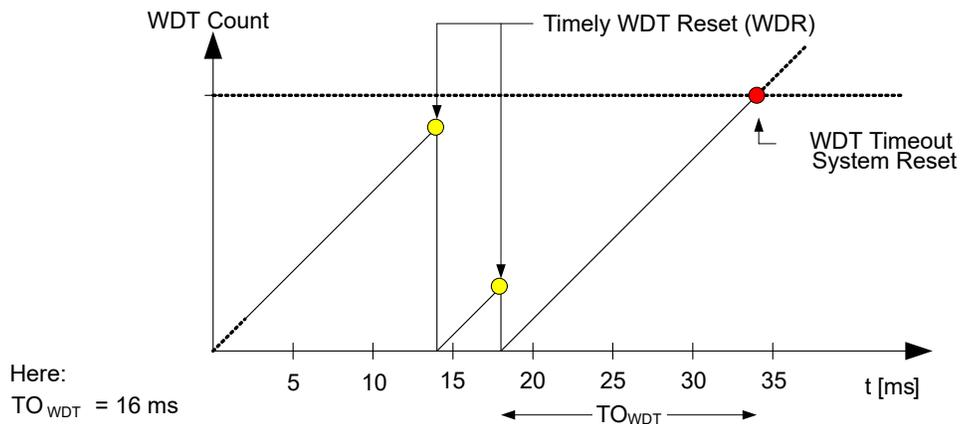
Normal mode is enabled as long as the WINDOW bit field in the Control A (WDT.CTRLA) register is  $0 \times 0$ .
