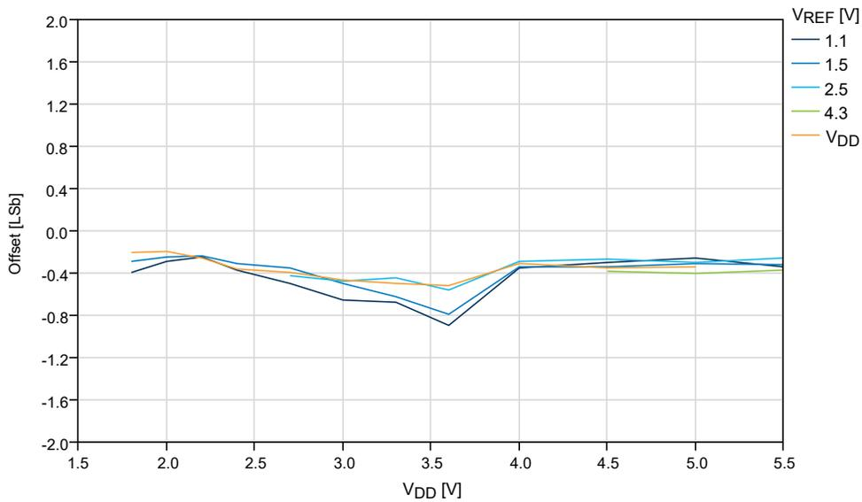
Figure 32-49. Offset Error vs.  $V_{REF}$  ( $V_{DD} = 5.0V$ ,  $f_{ADC} = 115$  ksp/s), REFSEL = Internal Reference
