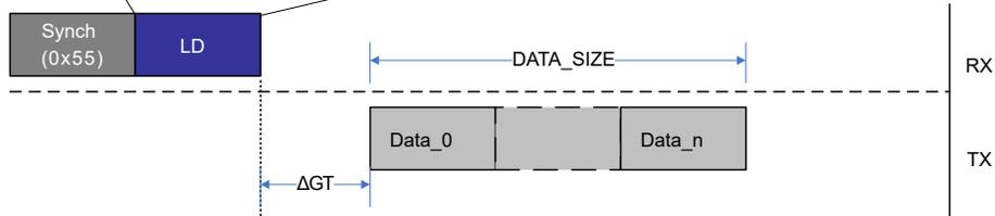
The figure above shows an example of a typical LD sequence, where the data are received after the Guard Time (GT) period. Loading data from the UPDI Pointer register follows the same transmission protocol.
