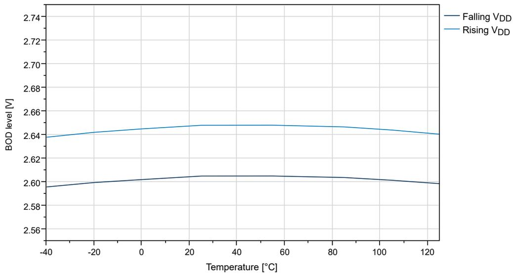
Figure 32-39. BOD Threshold vs. Temperature (Level 4.3V)
