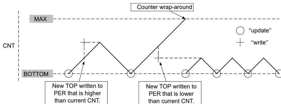
**With Buffering:** When double-buffering is used, the buffer can be written at any time and still maintain the correct operation. The TCA<sub>n</sub>.PER is always updated on the UPDATE condition, as shown for dual-slope operation in the figure below. This prevents wrap-around and the generation of odd waveforms.
