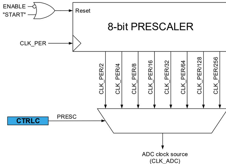
The ADC requires an input clock frequency between 50 kHz and 1.5 MHz for maximum resolution. If a lower resolution than ten bits is selected, the input clock frequency to the ADC can be higher than 1.5 MHz to get a higher sample rate.
