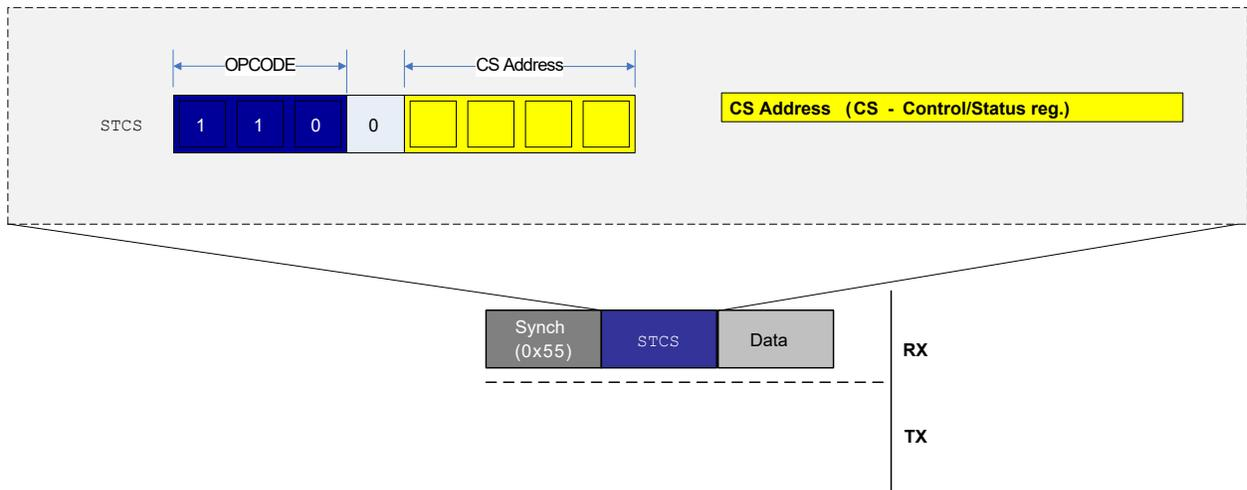
Figure 30-13 shows the data frame transmitted after the SYNCH character and the instruction frames. The STCS instruction byte can be immediately followed by the data byte. There is no response generated from the STCS instruction, as is the case for the ST and STS instructions.
