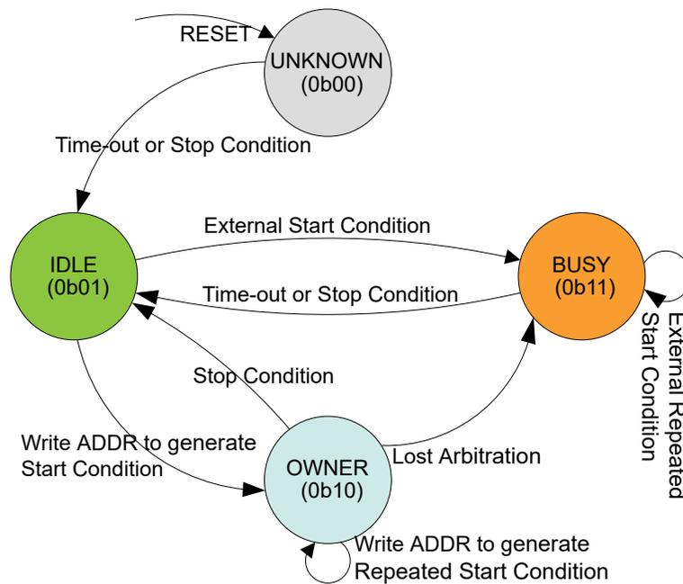
1. **Unknown:** The bus state machine is active when the TWI host is enabled. After the TWI host has been enabled, the bus state is Unknown. The bus state will also be set to Unknown after a system Reset is performed or after the TWI host is disabled.
