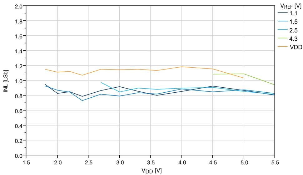
**Figure 32-47. INL vs.  $V_{REF}$  ( $V_{DD} = 5.0V$ ,  $f_{ADC} = 115$  ksp/s), REFSEL = Internal Reference**
