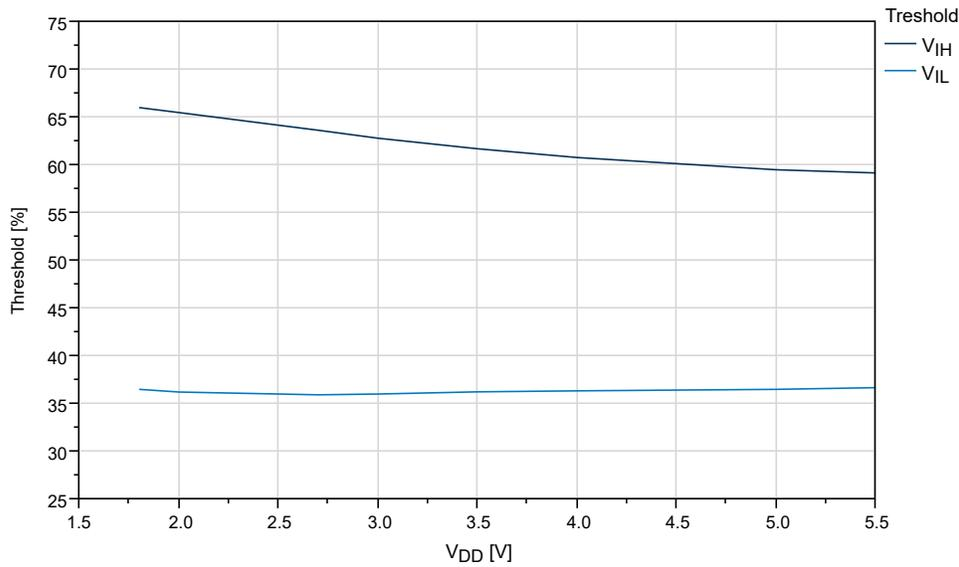
**Figure 32-17. I/O Pin Input Threshold Voltage vs.  $V_{DD}$  ( $V_{IH}$ )**
