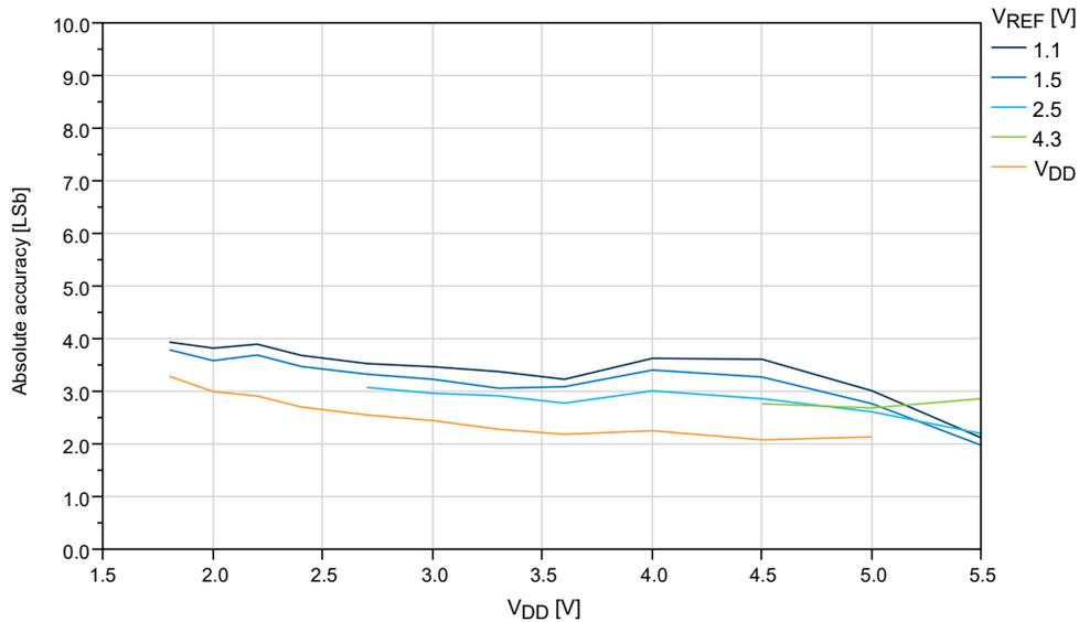
**Figure 32-41. Absolute Accuracy vs.  $V_{REF}$  ( $V_{DD} = 5.0V$ ,  $f_{ADC} = 115$  kps), REFSEL = Internal Reference**
