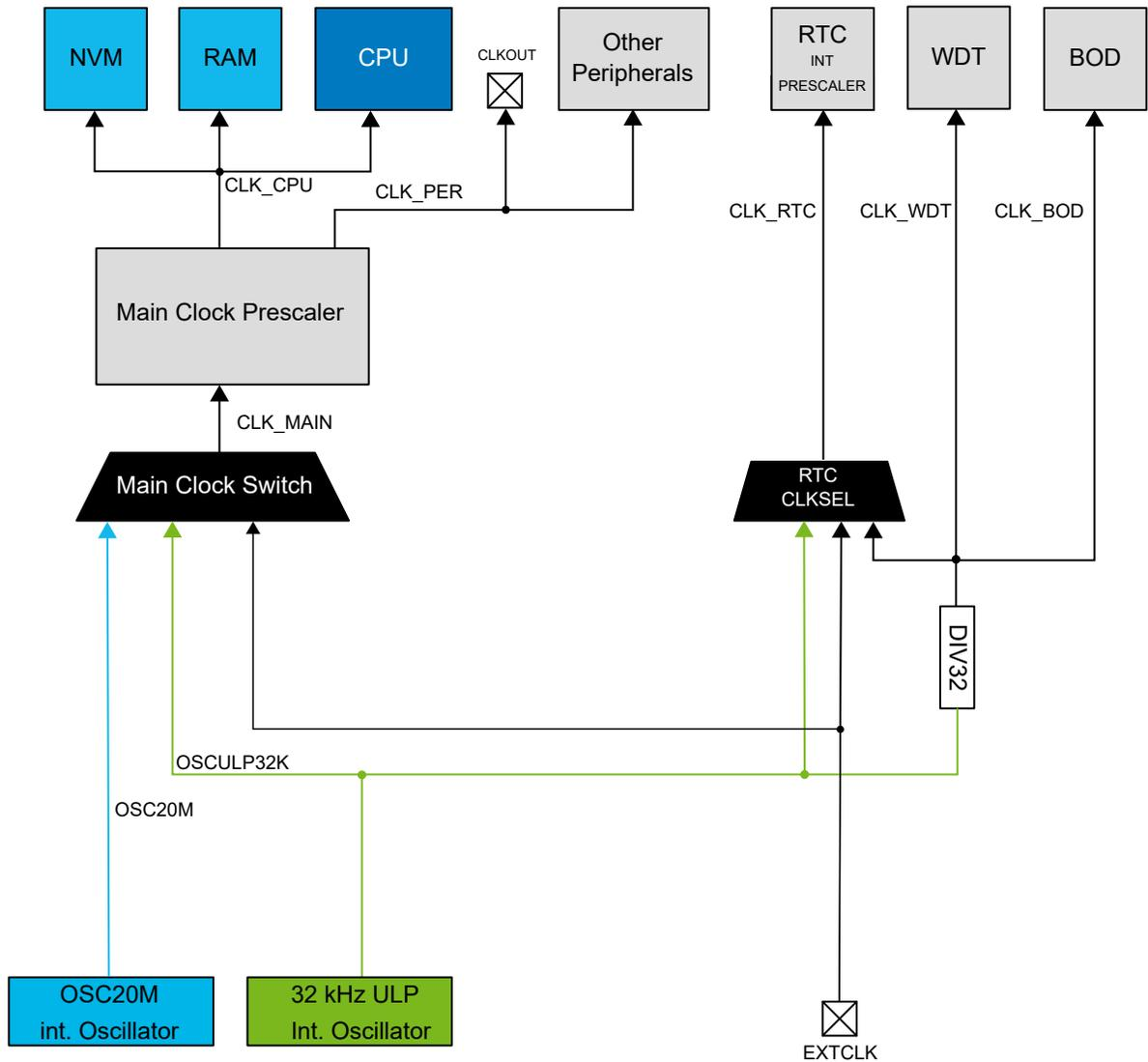
**Note:** The availability of the CLKOUT pin depends on the pin count of the device. See section 5. [I/O Multiplexing and Considerations](#) for an overview of which pins are available for each device represented in this data sheet.
