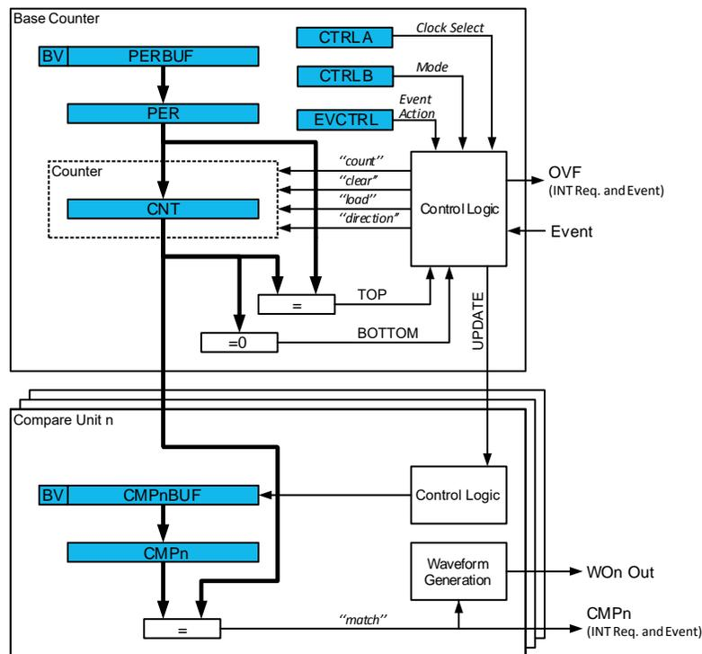
The Counter (TCA<sub>n</sub>.CNT) register, Period and Compare (TCA<sub>n</sub>.PER and TCA<sub>n</sub>.CMP<sub>n</sub>) registers, and their corresponding buffer registers (TCA<sub>n</sub>.PERBUF and TCA<sub>n</sub>.CMP<sub>n</sub>BUF) are 16-bit registers. All buffer registers have a Buffer Valid (BV) flag that indicates when the buffer contains a new value.
