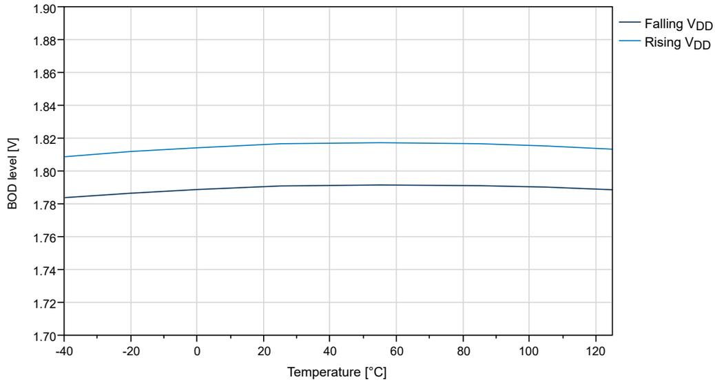
Figure 32-38. BOD Threshold vs. Temperature (Level 2.6V)
