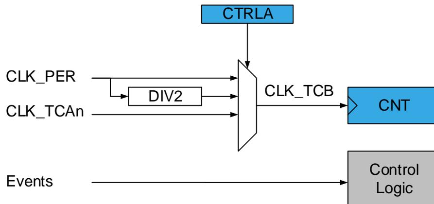
The Clock Select (CLKSEL) bit field in the Control A (TCBn.CTRLA) register selects one of the prescaler outputs directly as the clock (CLK\_TCB) input.
