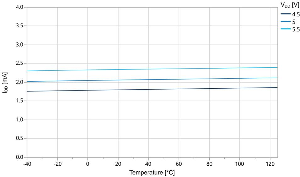
**Figure 32-9. Idle Supply Current vs.  $V_{DD}$  ( $f = 32.768$  kHz OSCULP32K)**
