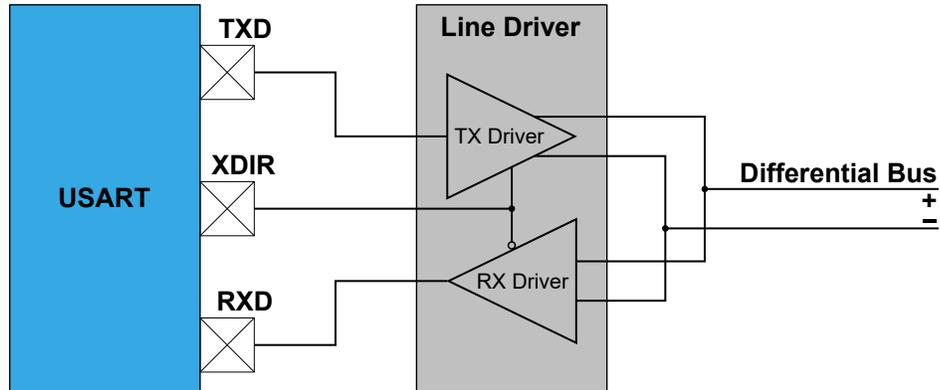
The XDIR pin goes high one baud clock cycle in advance of data being shifted out to allow some guard time to enable the external line driver. The XDIR pin will remain high for the complete frame, including Stop bit(s).
