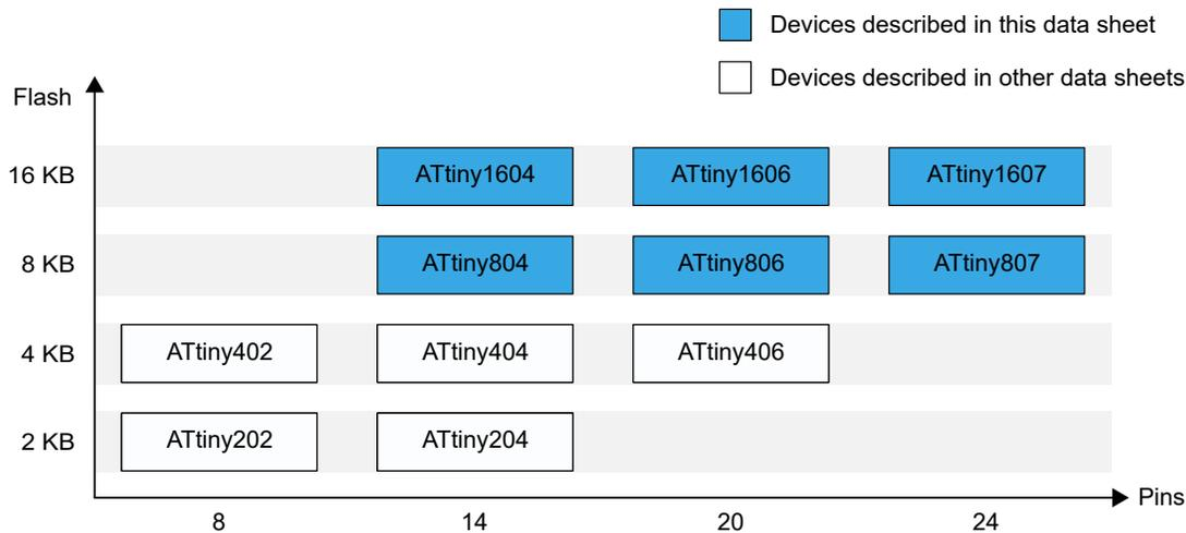
Devices with different Flash memory sizes typically also have different SRAM and EEPROM.
