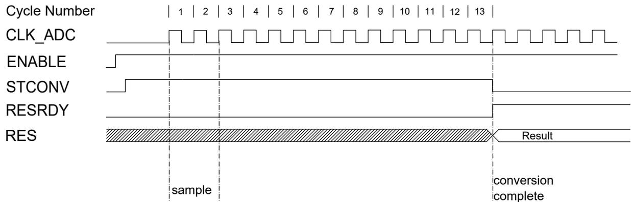
Both sampling time and sampling length can be adjusted using the Sample Delay (SAMPDLY) bit field in the Control D (ADCn.CTRLD) register and the Sample Length (SAMPLN) bit field in the Sample Control (ADCn.SAMPCTRL) register. Both of these control the ADC sampling time in some CLK\_ADC cycles. This allows sampling of high-impedance sources without relaxing conversion speed. See the register description for further information. Total sampling time is given by:
