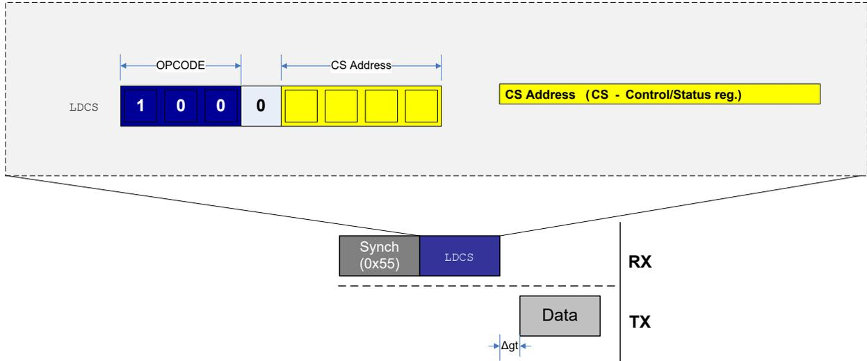
Figure 30-12 shows a typical example of `LDCS` data transmission. A data byte from the `LDCS` is transmitted from the UPDI after the guard time is completed.
