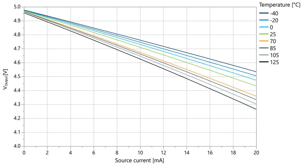
**Figure 32-26. I/O Pin Output Voltage vs. Source Current ( $T = 25^{\circ}C$ )**
