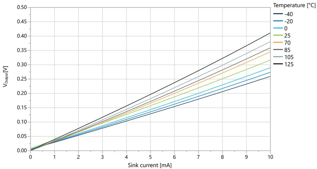
Figure 32-21. I/O Pin Output Voltage vs. Sink Current ( $V_{DD} = 5.0V$ )
