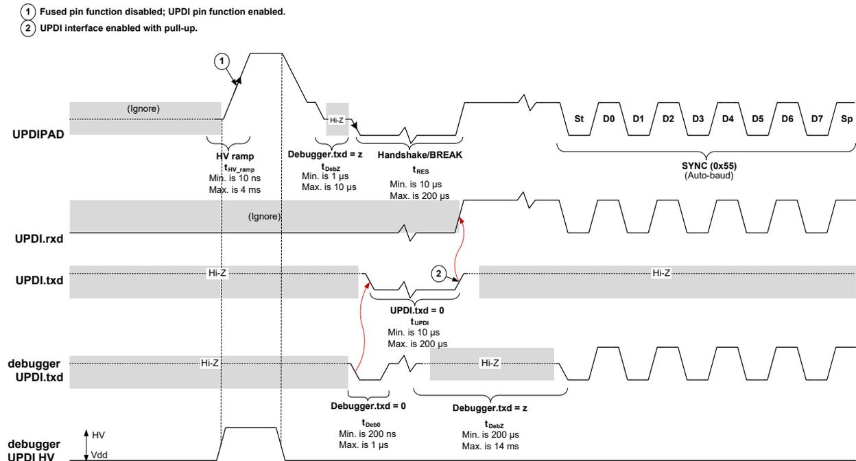
When enabled by an HV pulse, only a POR will disable the UPDI configuration on the  $\overline{\text{RESET}}$  pin and restore the default setting. If issuing a UPDI Disable command through the UPDIDIS bit in UPDI.CTRLB, the UPDI will be reset, and the clock request will be canceled, but the  $\overline{\text{RESET}}$  pin will remain in UPDI configuration.
