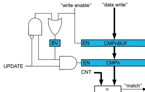
Both the TCA<sub>n</sub>.CMP<sub>n</sub> and TCA<sub>n</sub>.CMP<sub>n</sub>BUF registers are available as I/O registers. This allows the initialization and bypassing of the buffer register and the double-buffering function.
