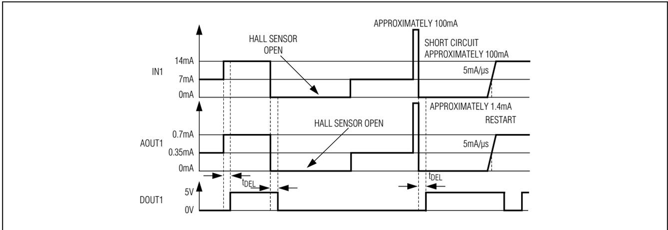
Figure 1. Timing Diagram
