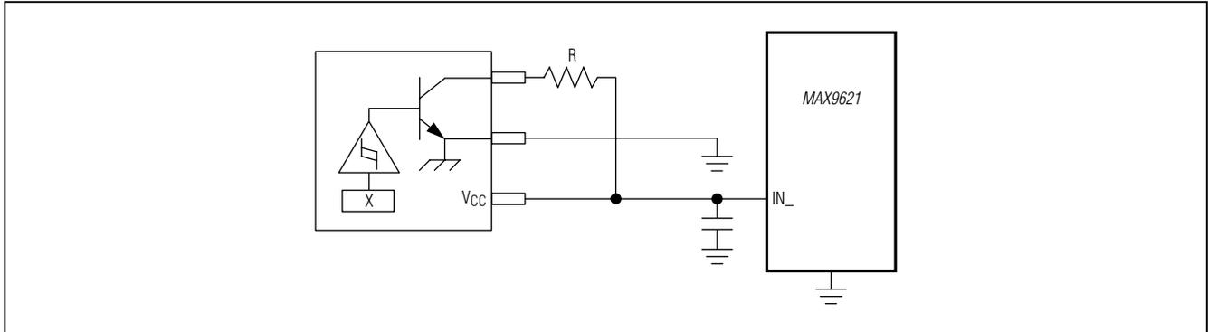
Figure 5. 3-Wire Hall-Effect Switches Configured as 2-Wire
