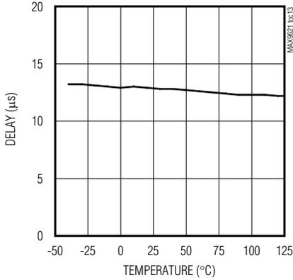
**DELAY DIFFERENCE BETWEEN CHANNELS vs. TEMPERATURE**
