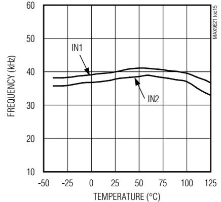
**IN\_ PULSE LENGTH REJECTED BY FILTER TO DOUT\_ vs. TEMPERATURE**
