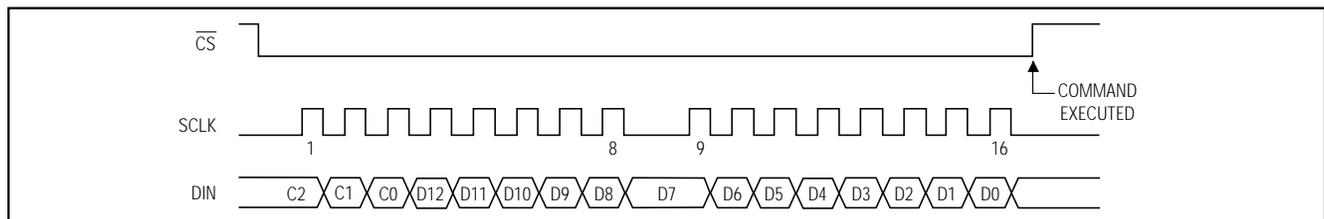
Figure 6. Serial-Interface Timing
