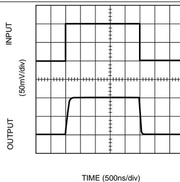
Figure 24. Non-Inverting Small Signal Pulse Response
