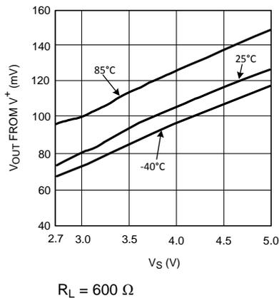
Figure 5. Output Positive Swing vs Supply Voltage
