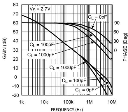
**Figure 17. Open Loop Frequency Response vs  $C_L$**
