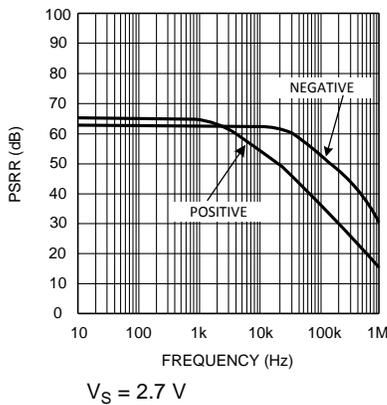
Figure 11. PSRR vs Frequency
