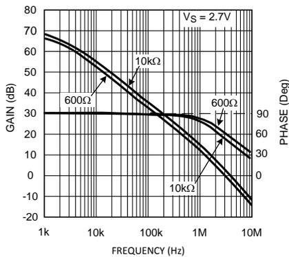
**Figure 15. Open Loop Frequency Response vs  $R_L$**
