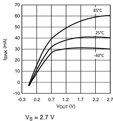
Figure 9. Sinking Current vs Output Voltage
