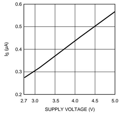
Figure 2. Supply Current vs Supply Voltage (Shutdown)
