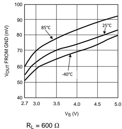
Figure 6. Output Negative Swing vs Supply Voltage
