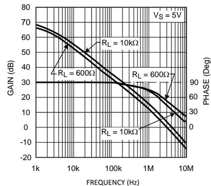
**Figure 16. Open Loop Frequency Response vs  $R_L$**
