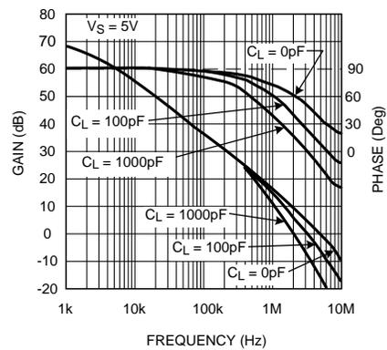
**Figure 18. Open Loop Frequency Response vs  $C_L$**
