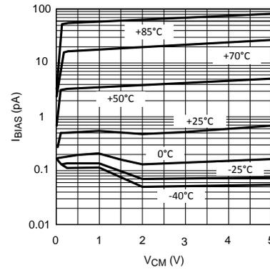
Figure 4.  $I_B$  vs  $V_{CM}$  Over Temperature
