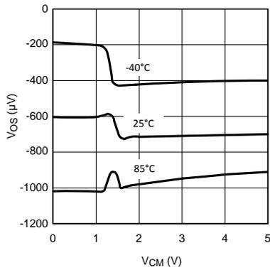
Figure 3.  $V_{OS}$  vs  $V_{CM}$
