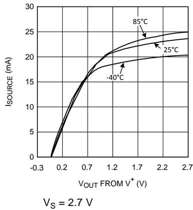
Figure 7. Sourcing Current vs Output Voltage
