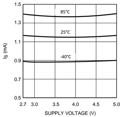
Figure 1. Supply Current Per Channel vs Supply Voltage
