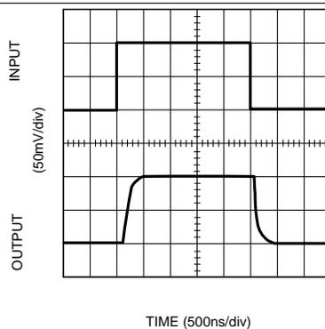
Figure 23. Non-Inverting Small Signal Pulse Response
