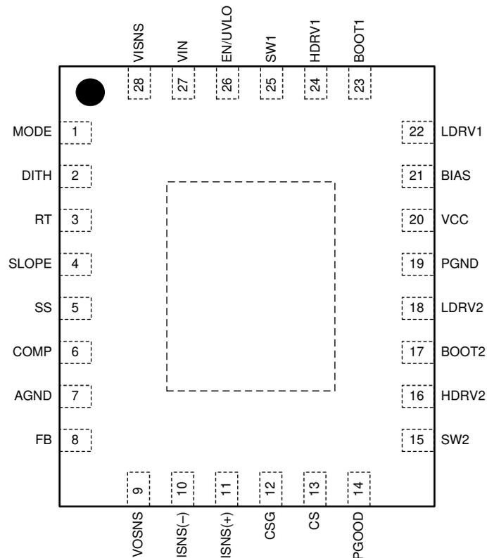
**Figure 5-1. QFN-28 RHF Package Top View**
