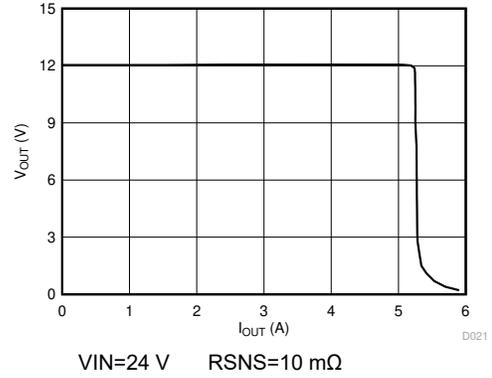
**Figure 6-20. Constant Current Constant Voltage (CCCV) Operation**
