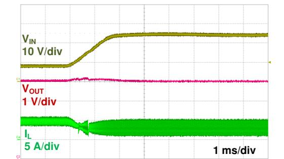
VIN=8 V to 24 V VOUT=12 V IOUT=3A
