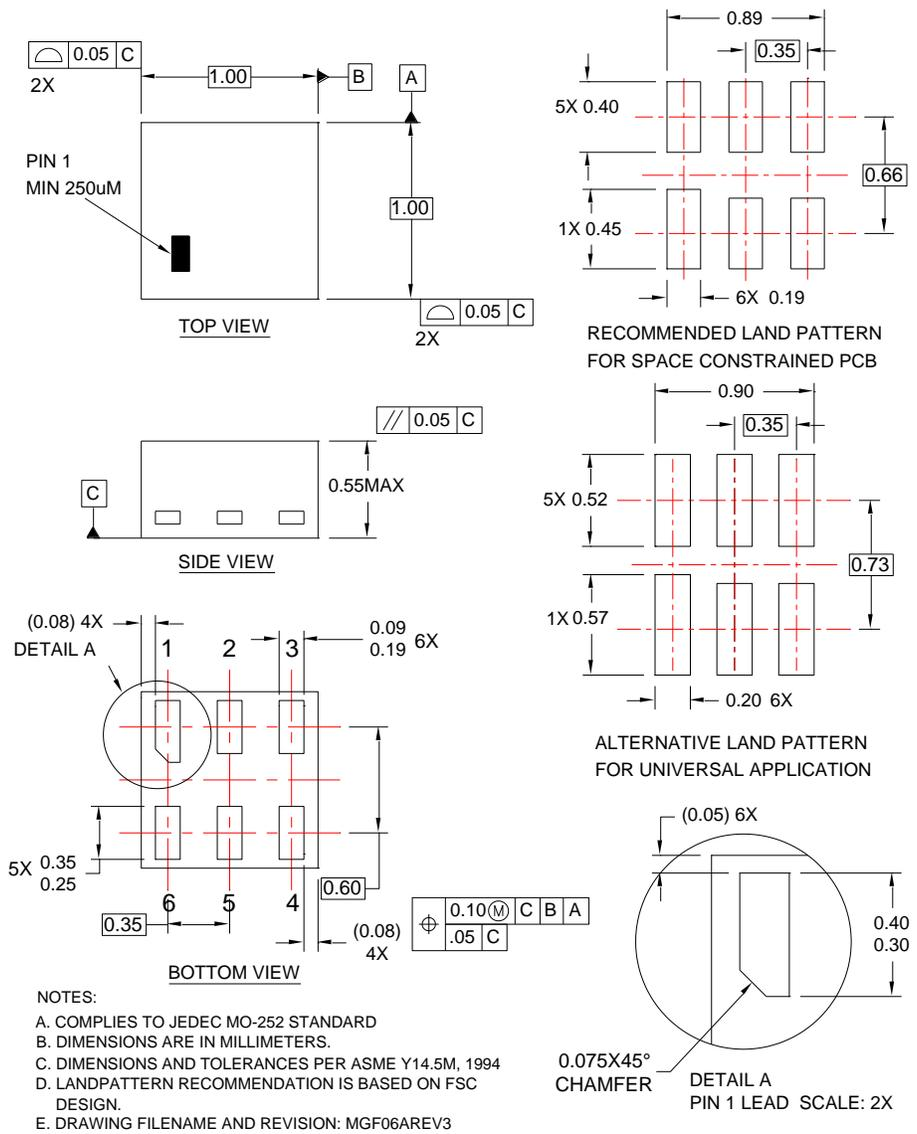
**Figure 10. 6-Lead, MicroPak2™, 1x1mm Body, .35mm Pitch**
