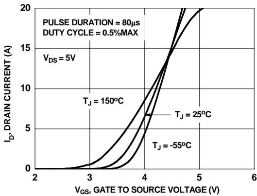
Figure 5. Transfer Characteristics
