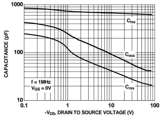
**Figure 22. Capacitance vs Drain to Source Voltage**
