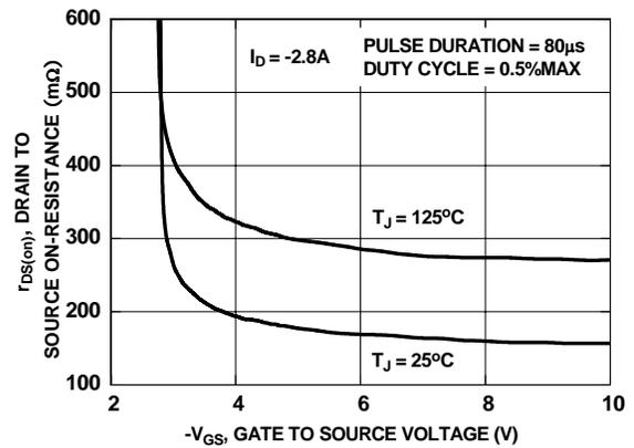
Figure 18. On-Resistance vs Gate to Source Voltage
