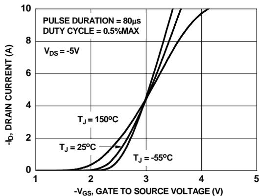
Figure 19. Transfer Characteristics
