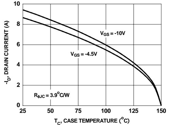
**Figure 24. Maximum Continuous Drain Current vs Case Temperature**
