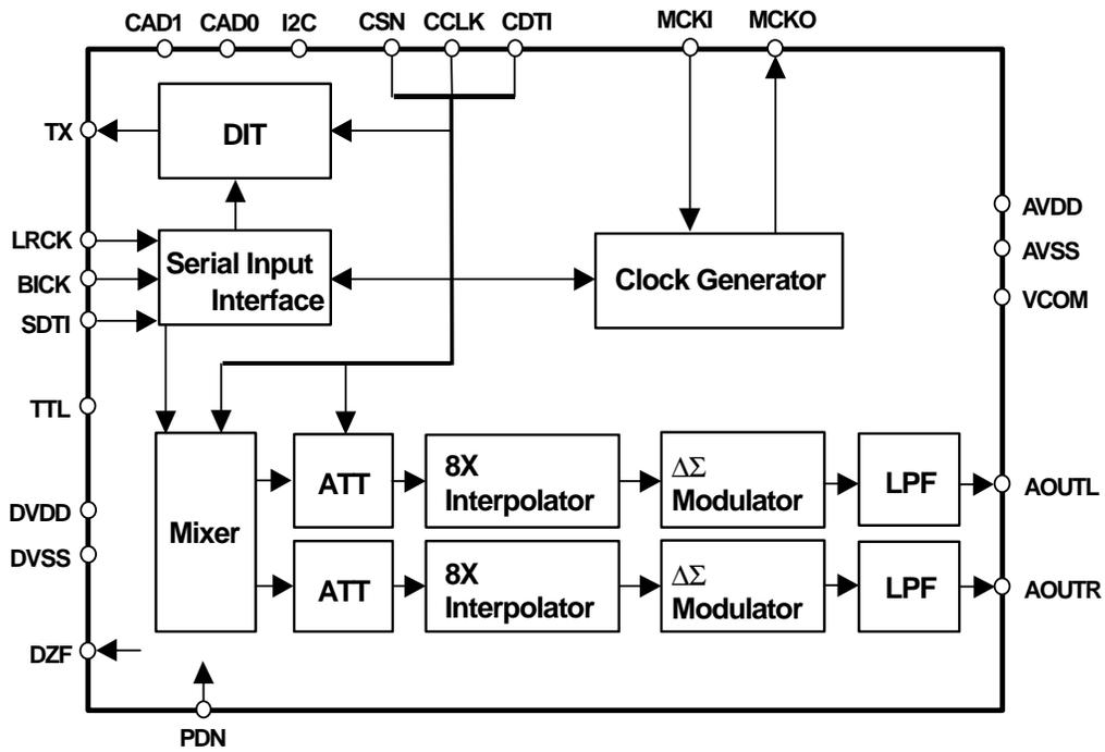
Figure 1. 3-wire Serial Control Mode (I2C = "L")
