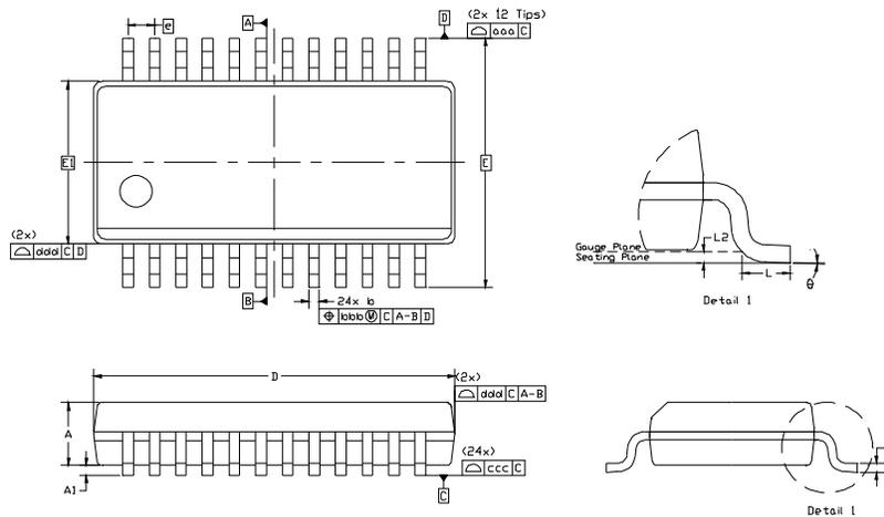
**Figure 16. 24-Pin SSOP**
