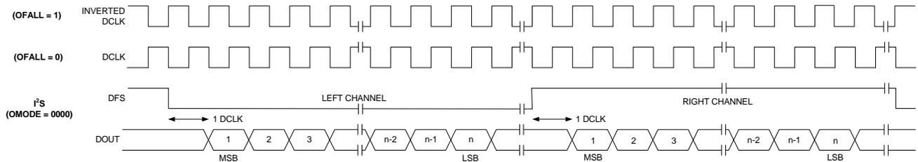
**Figure 10. I<sup>2</sup>S Digital Audio Format**
