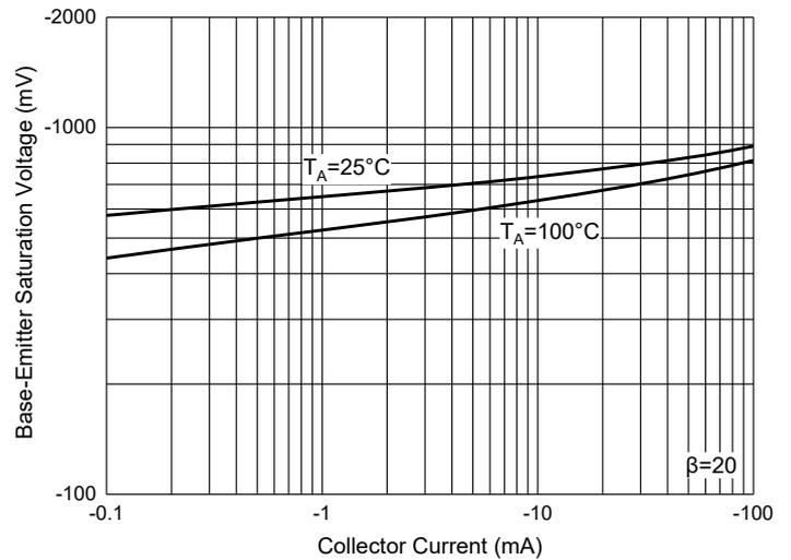
Fig. 5 - Base-Emitter Voltage Characteristics
