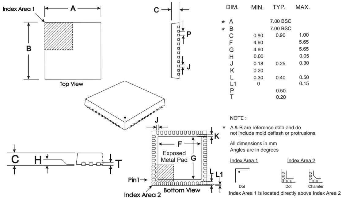
Figure 33 Mechanical Outline of 48-pin VQFN (Q3)
