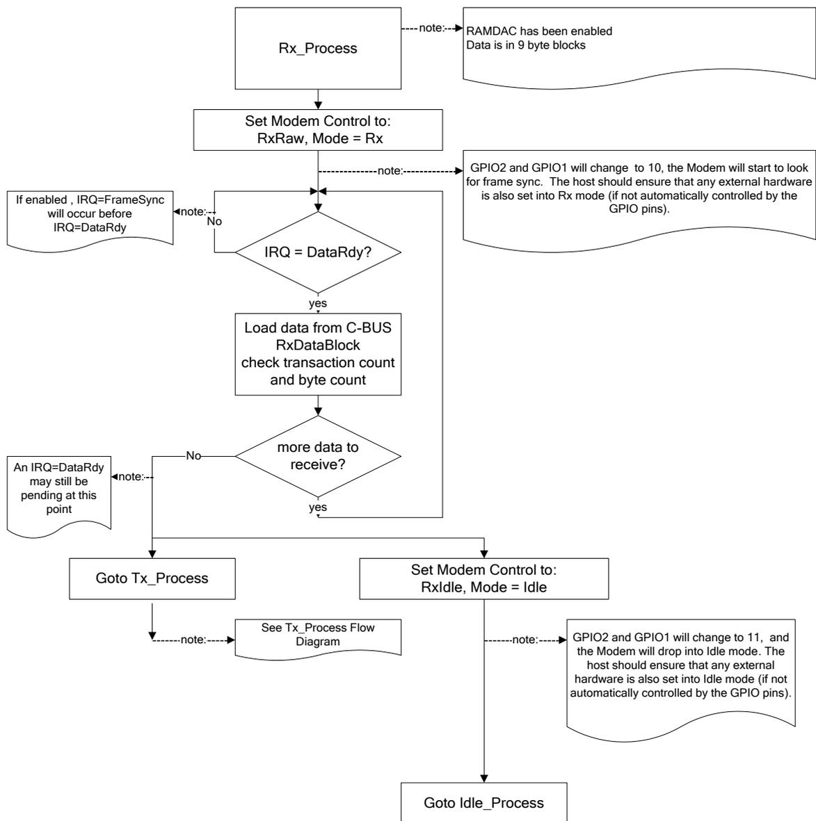
Figure 22 Rx Data Flow (Raw Data Mode)
