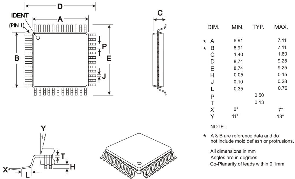
Figure 32 Mechanical Outline of 48-pin LQFP (L4)
