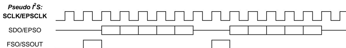
**Figure 19 I<sup>2</sup>S Mode Support**
