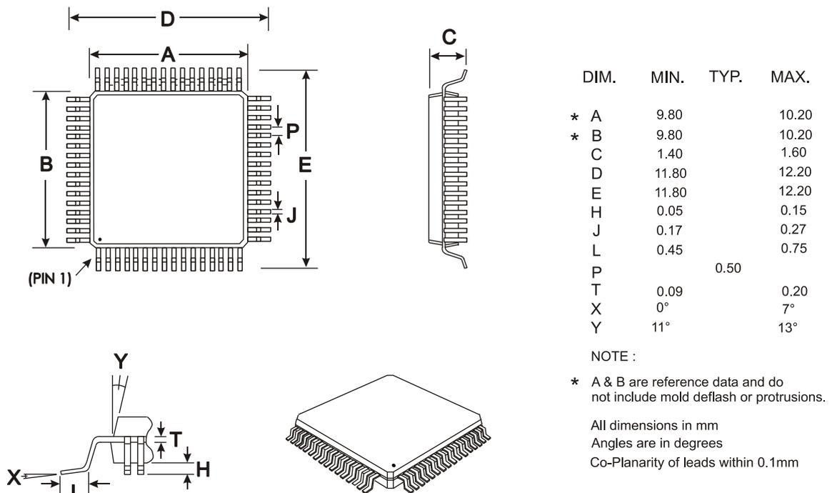
Figure 31 Mechanical Outline of 64-pin LQFP (L9)
