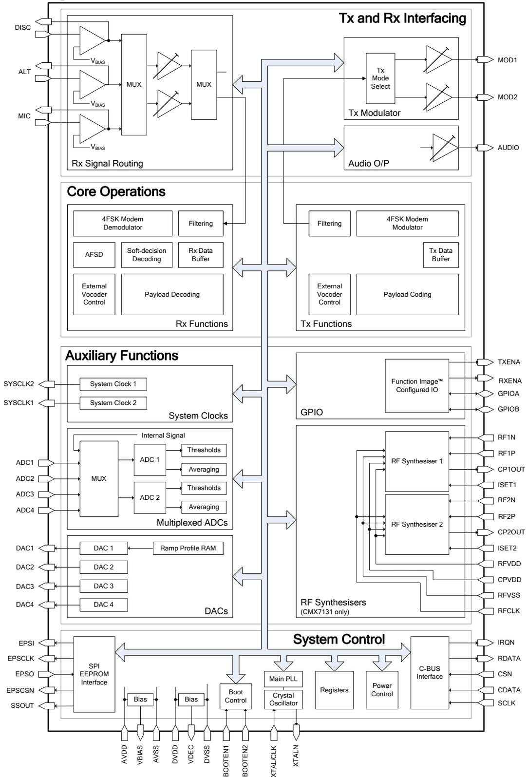
Figure 1 Block Diagram
