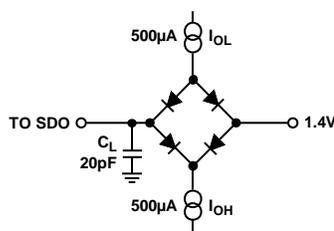
Figure 2. Load Circuit for Digital Interface Timing
