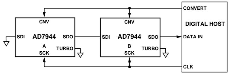
Figure 34. Chain Mode Without Busy Indicator Connection Diagram
