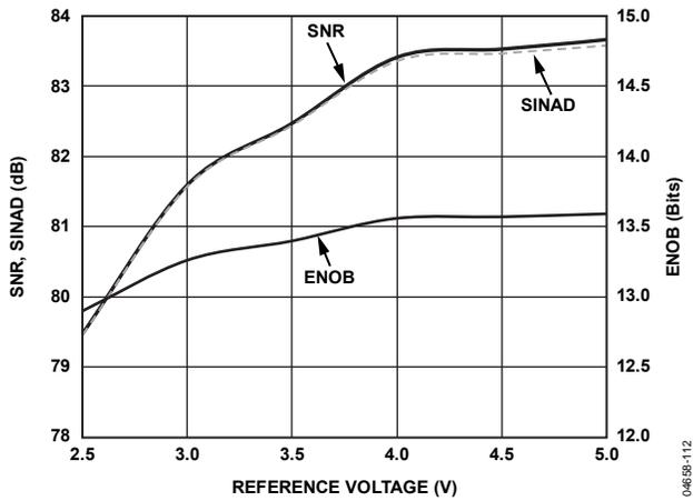
Figure 12. SNR, SINAD, and ENOB vs. Reference Voltage
