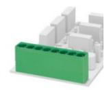
PCB headers, nominal current: 76 A, number of positions: 2, pitch: 10.16 mm, color: green, contact surface: Silver, mounting: Wave soldering, The nominal current of 76 A applies in connection with connectors from the PC 16 family. 41 A are reached in connection with PC 6 connectors (50 A in accordance with UL).
