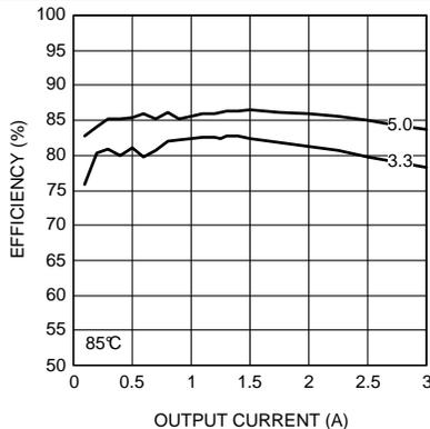
**Figure 17. Efficiency 36-V Input at 85°C**
