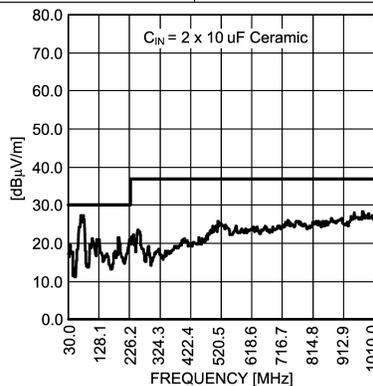
Figure 29. Radiated Emissions (EN 55022 Class B)
