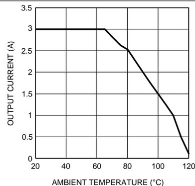
Figure 28. Thermal Derating Curve
