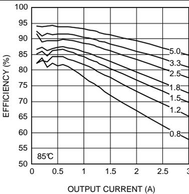
**Figure 11. Efficiency 8-V Input at 85°C**
