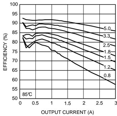
**Figure 13. Efficiency 12-V Input at 85°C**
