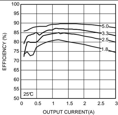
**Figure 5. Efficiency 24-V Input at 25°C**
