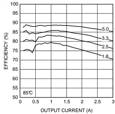
**Figure 15. Efficiency 24-V Input at 85°C**
