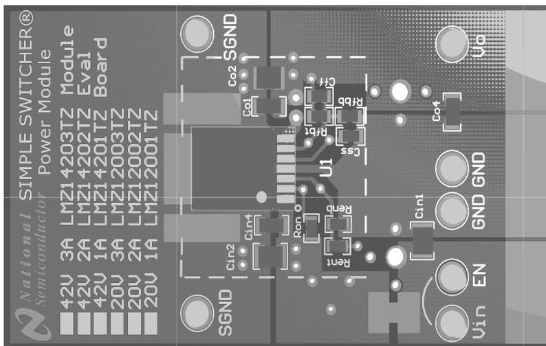
Figure 32. EVM Board Layout - Top View
