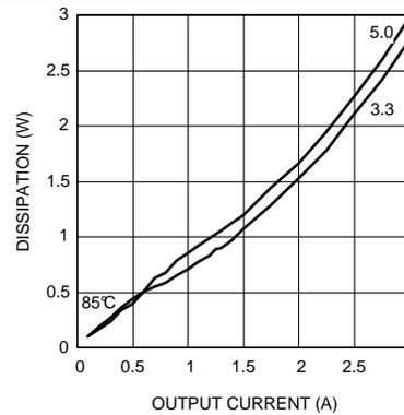
**Figure 18. Dissipation 36-V Input at 85°C**
