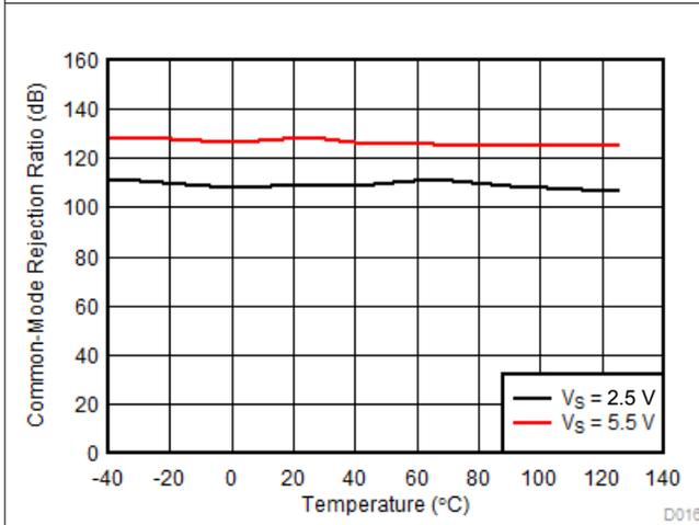
**Figure 6-11. DC CMRR vs Temperature**
