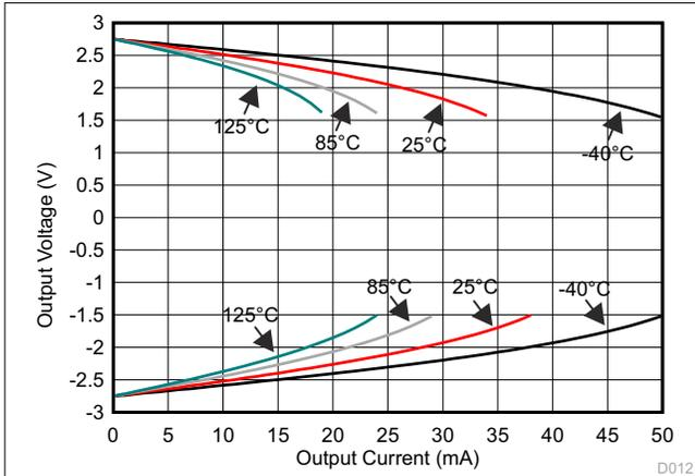
**Figure 6-7. Output Voltage vs Output Current (Claw)**
