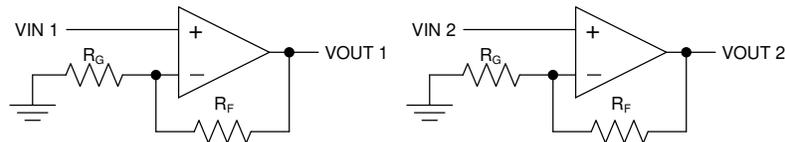
**Figure 10-1. Schematic Representation**
