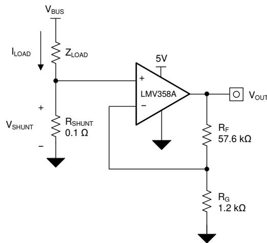
Figure 8-1. LMV3xxA in a Low-Side, Current-Sensing Application
