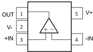
Figure 5-1. LMV321A DBV Package, 5-Pin SOT-23 (Top View)
