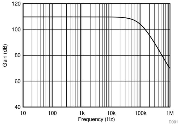
**Figure 8-4. Photodiode Amplifier Circuit AC Gain Results**
