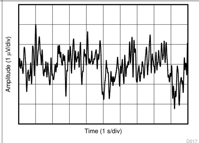
**Figure 6-12. 0.1 Hz to 10 Hz Integrated Voltage Noise**
