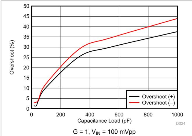
**Figure 6-19. Small Signal Overshoot vs Capacitive Load**
