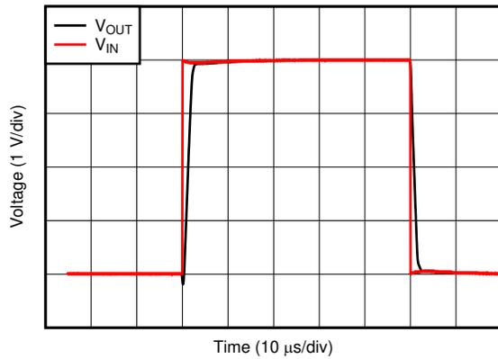
$G = 1$ ,  $V_{IN} = 4 V_{PP}$ ,  $C_L = 10\text{ pF}$
