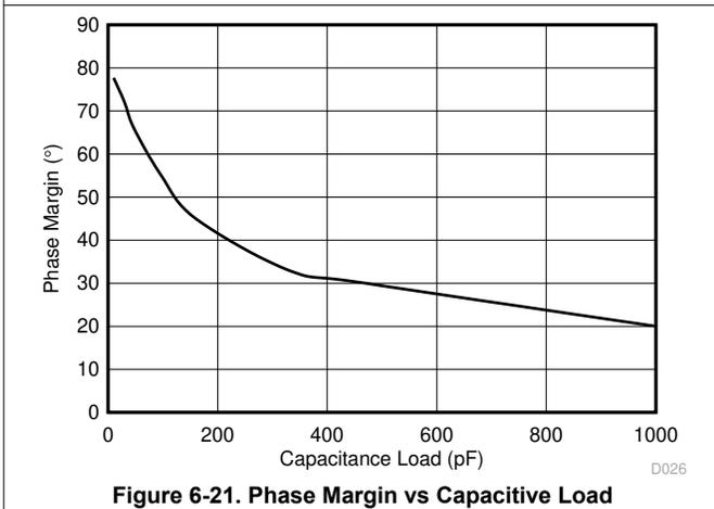
**Figure 6-21. Phase Margin vs Capacitive Load**
