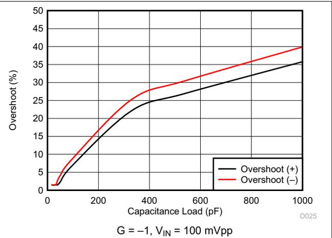
**Figure 6-20. Small Signal Overshoot vs Capacitive Load**
