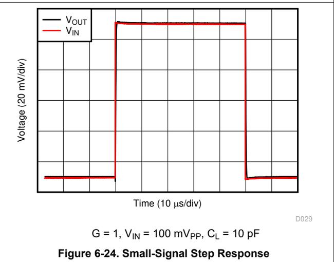
**Figure 6-24. Small-Signal Step Response**
