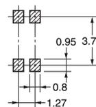
Unless otherwise specified, the dimensional tolerance is  $\pm 0.1$  mm.
