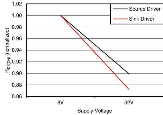
**Figure 6-4.  $R_{DS(ON)}$  vs  $V_{BB}$  (Normalized to  $V_{BB} = 8$  V)**
