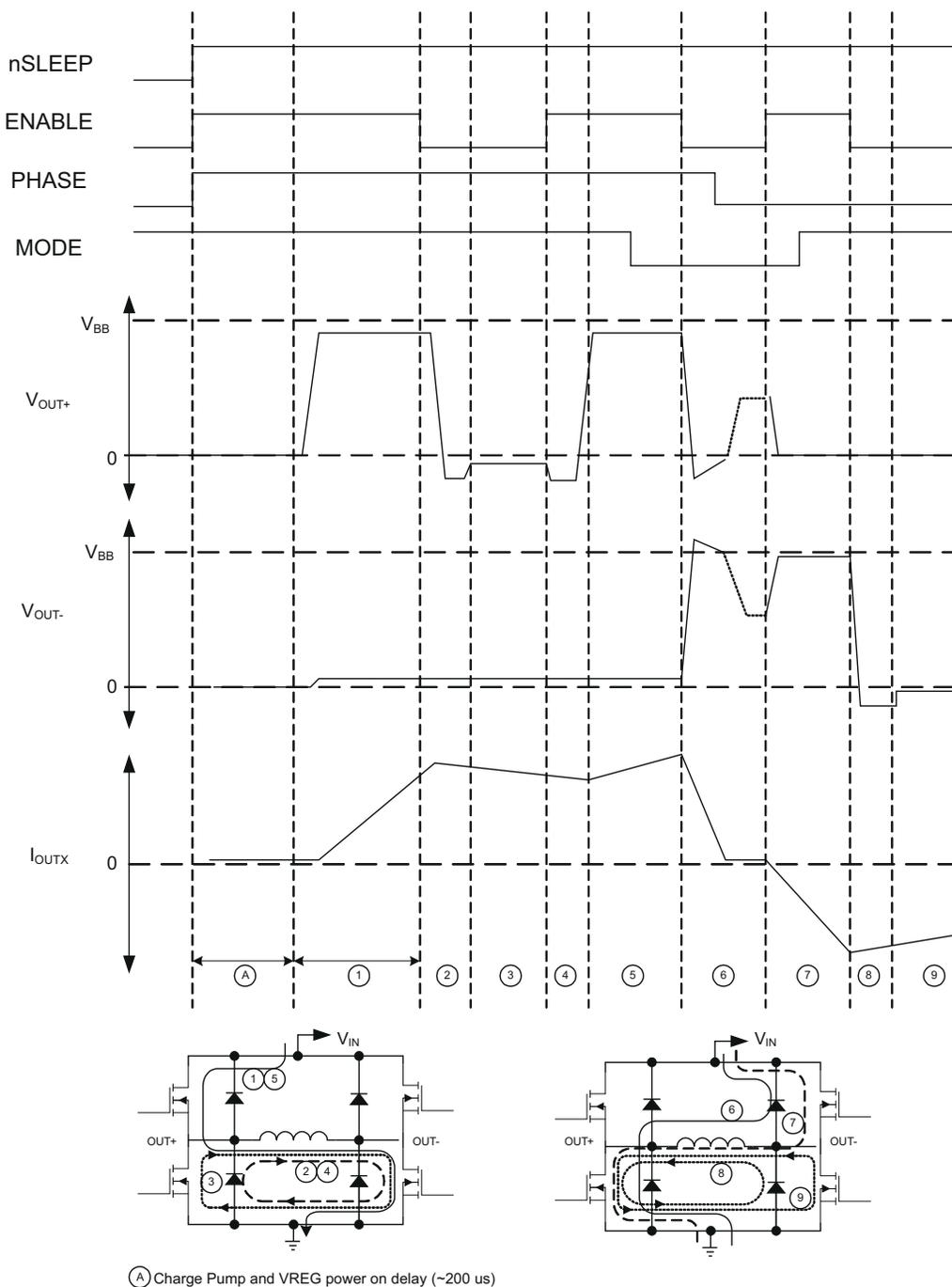
**Figure 6-1. PWM Control Timing**
