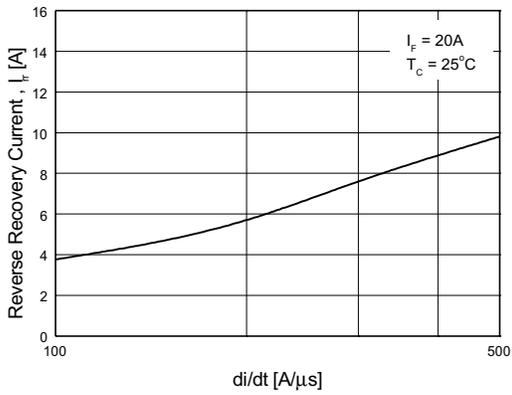
**Figure 5. Typical Reverse Recovery Current vs. di/dt**
