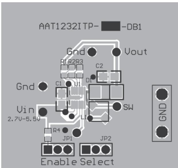
**Figure 4: AAT1232 Evaluation Board Top Side Layout.**
