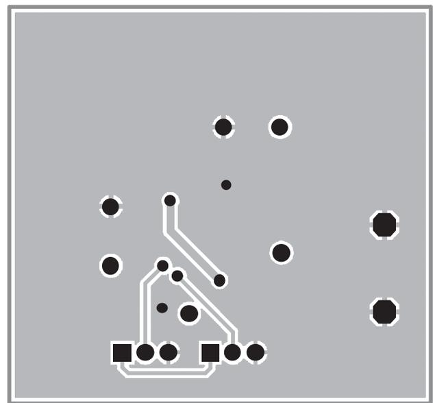
**Figure 5: AAT1232 Evaluation Board Bottom Side Layout.**
