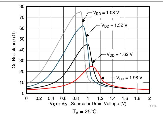
Figure 4. On-Resistance vs Source or Drain Voltage
