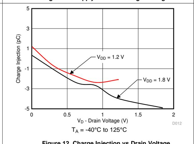
Figure 12. Charge Injection vs Drain Voltage
