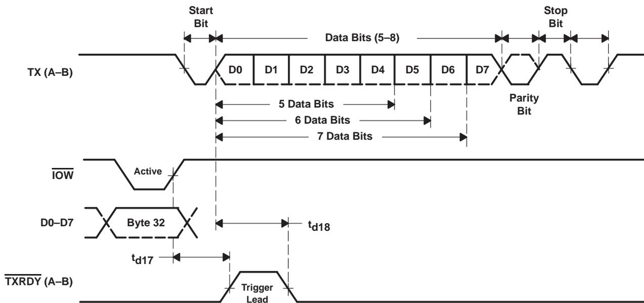
Figure 19. Transmit Ready Timing in FIFO Mode
