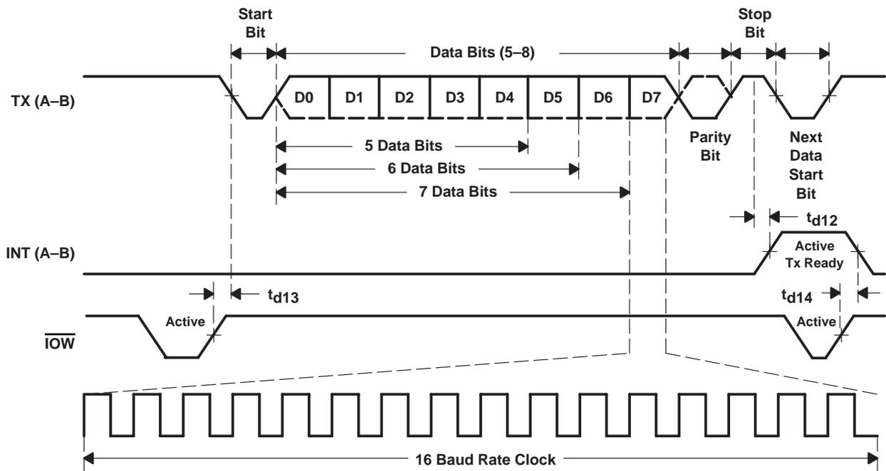
Figure 17. Transmit Timing
