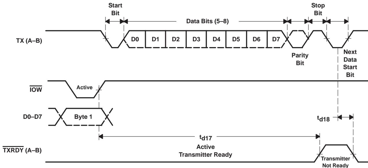
Figure 18. Transmit Ready Timing in None FIFO Mode
