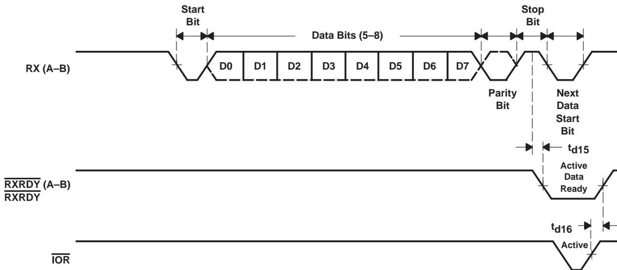
Figure 15. Receive Ready Timing in None FIFO Mode
