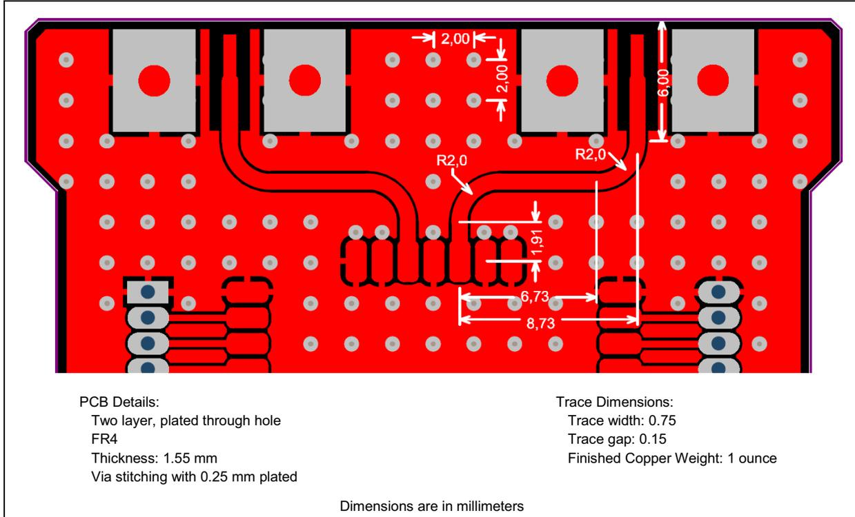
FIGURE 5-2: RF TRACE ROUTING (BOTTOM LAYER)
