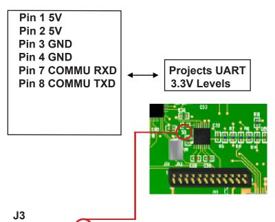
Note: Cut Trace across SD and Jumper "D" side to C38 "8" side GND to take the RS232 Tranceiver out of circuit.
