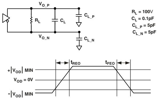
Figure 17. Link Ports—Differential Output Signals Transition Time
