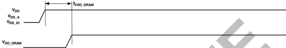
Figure 10. Power-Up Timing
