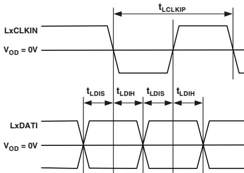
Figure 23. Link Ports—Data Input Setup and Hold<sup>1</sup>
