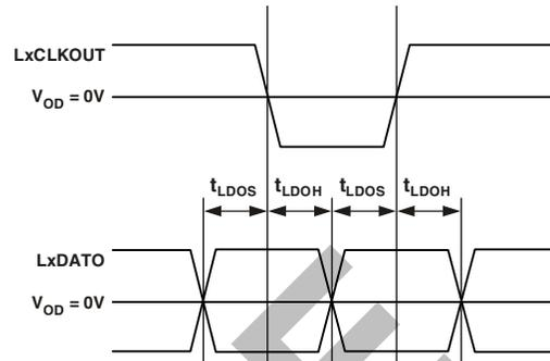
Figure 18. Link Ports—Data Output Setup and Hold<sup>1</sup>
