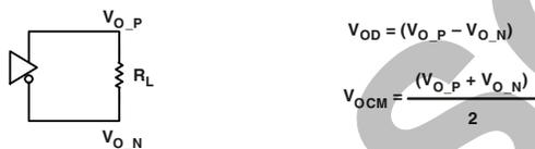
Figure 14. Link Ports—Transmit Electrical Characteristics
