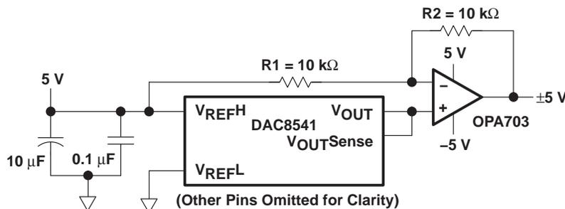
Figure 34. Bipolar Operation With the DAC8541
