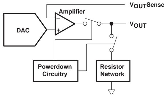
Figure 31. Output Stage During Power Down (High-Impedance)
