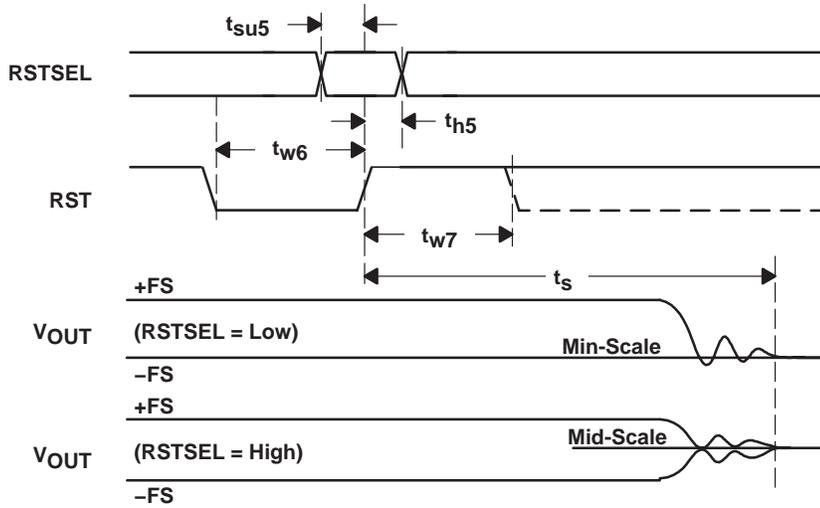
Figure 2. Reset Timing
