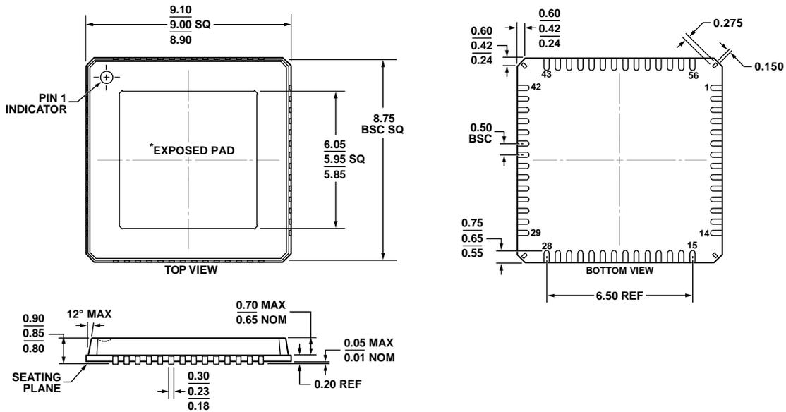
\*FOR PROPER CONNECTION OF THE EXPOSED PAD, REFER TO THE PIN CONFIGURATION AND FUNCTION DESCRIPTIONS SECTION OF THIS DATA SHEET.
