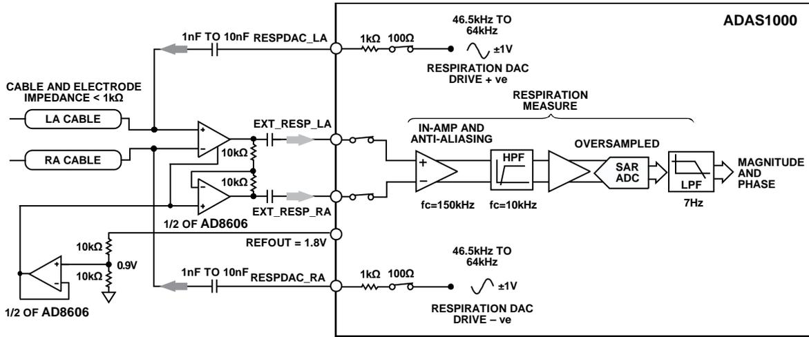
Figure 71. Respiration Using External Capacitor and External Amplifiers
