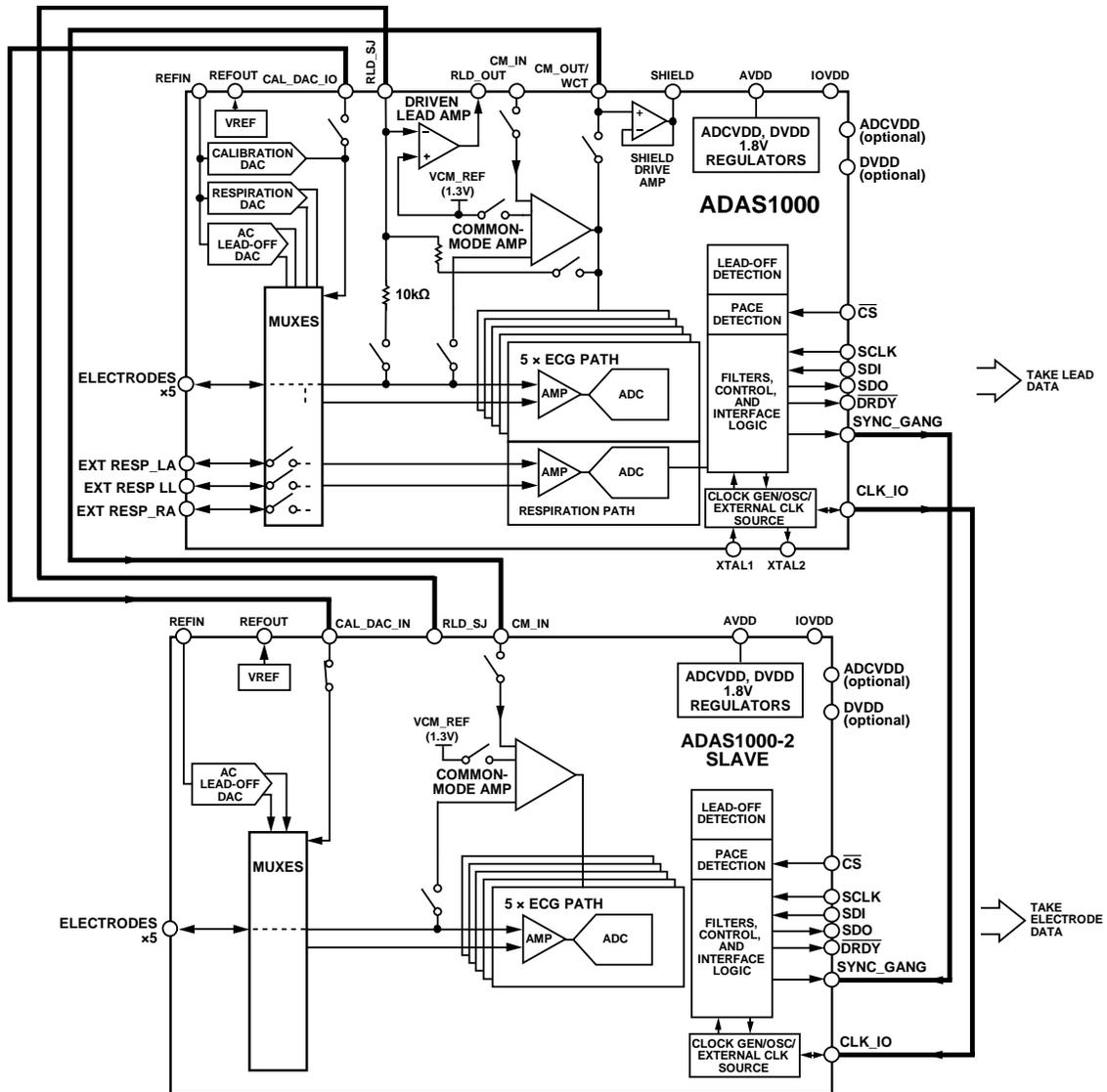
Figure 77. Configuring Multiple Devices to Extend Number of Electrodes/Leads
