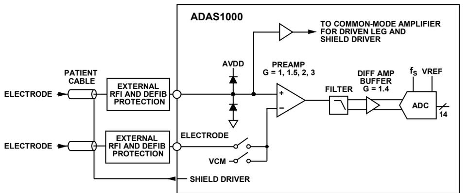
Figure 56. Simplified Schematic of a Single ECG Channel
