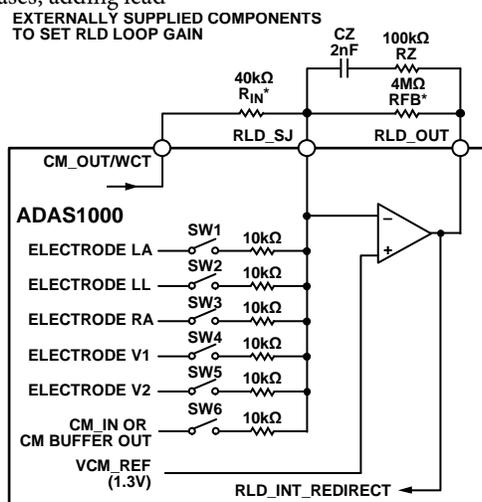
\*EXTERNAL RESISTOR R<sub>IN</sub> IS OPTIONAL. IF DRIVING RLD FROM THE ELECTRODE PATHS, THEN THE SERIES RESISTANCE WILL CONTRIBUTE TO THE R<sub>IN</sub> IMPEDANCE. WHERE SW1 TO SW5 ARE CLOSED, R<sub>IN</sub> = 2kΩ. RFB SHOULD BE CHOSEN ACCORDINGLY FOR DESIRED RLD LOOP GAIN.
