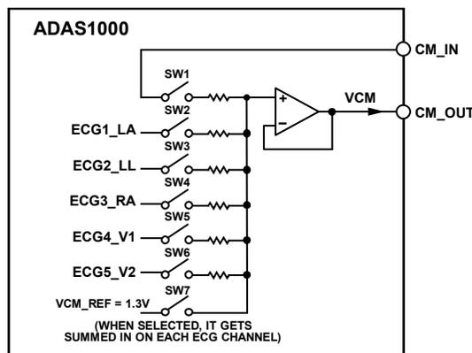
Figure 66. Common-Mode Generation Block
