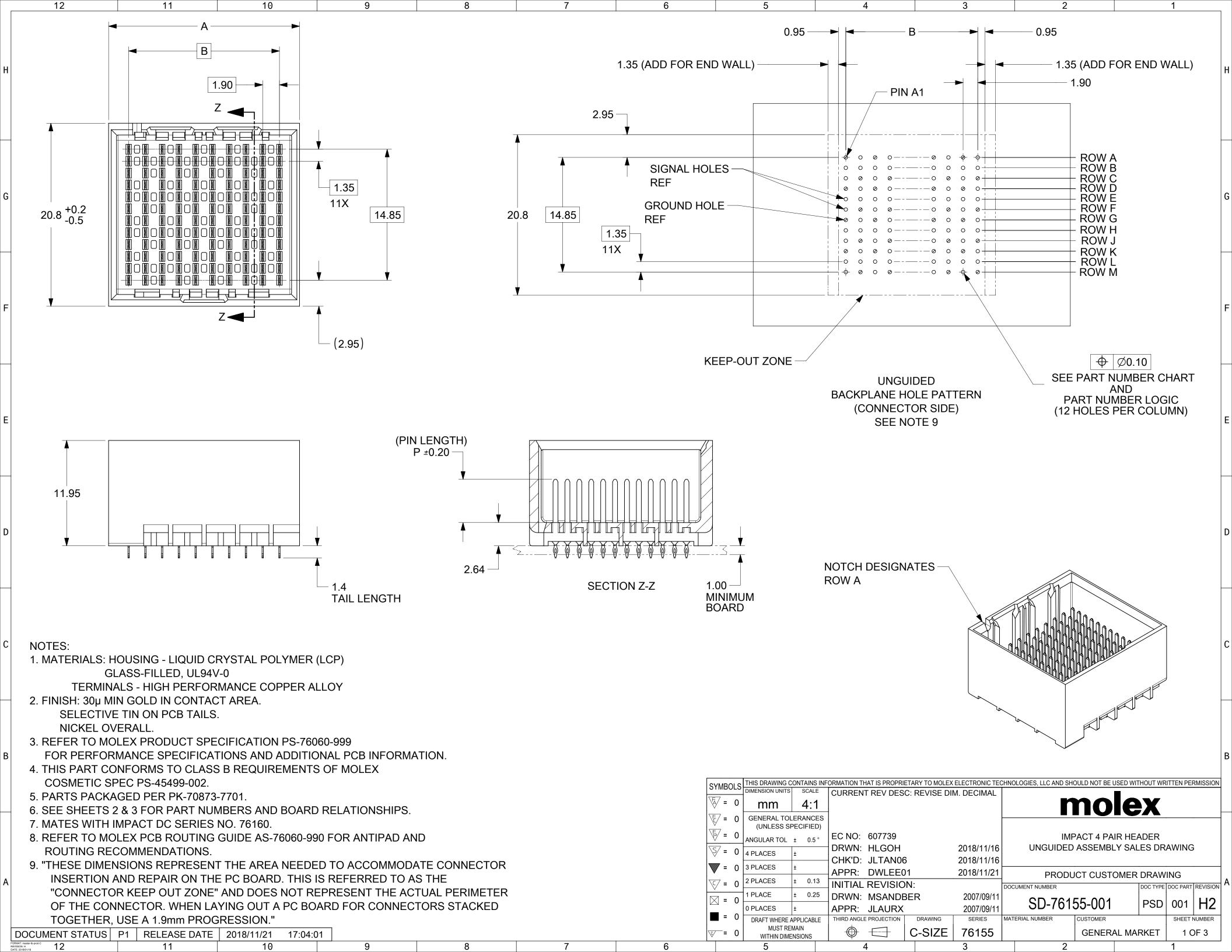
2 11 10 8 6 5 4 1 12 PART NUMBER TABLE MATERIAL NUMBER # OF COLUMNS # OF DIFF PAIR DIM "A" DIM "B" DUAL 76155-\*32\* 24 14.1 9.50 **DUAL END END WALL** 13.30 76155-\*82\* 32 17.9 8 **WALL OPTION OPTION** 76155-\*12\* 21.7 17.10 10 40 76155-\*62\* 16 33.1 28.50 64
