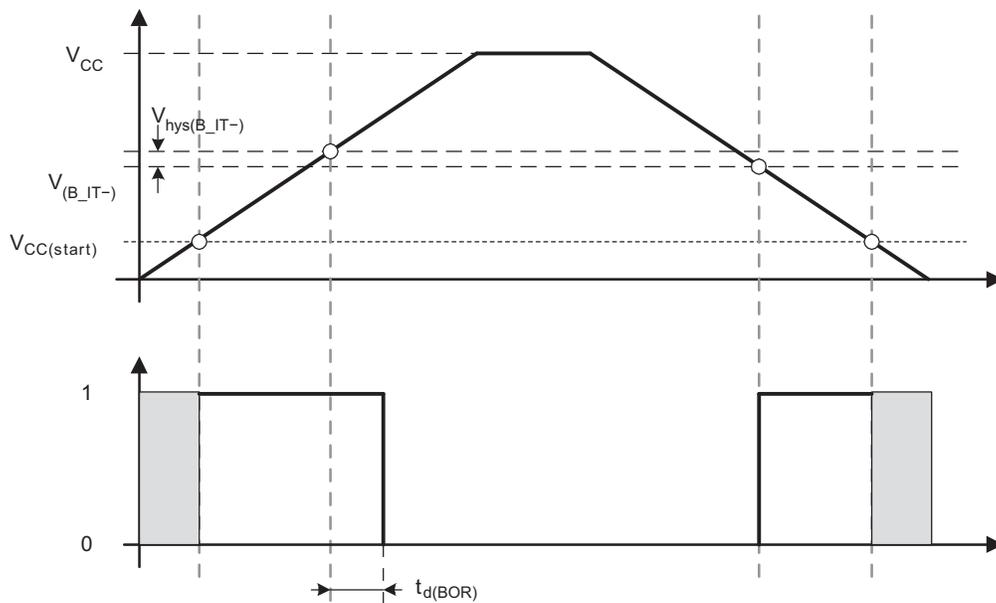
Figure 5-12. POR and BOR vs Supply Voltage
