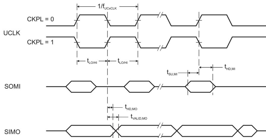
**Figure 5-17. SPI Master Mode, CKPH = 1**
