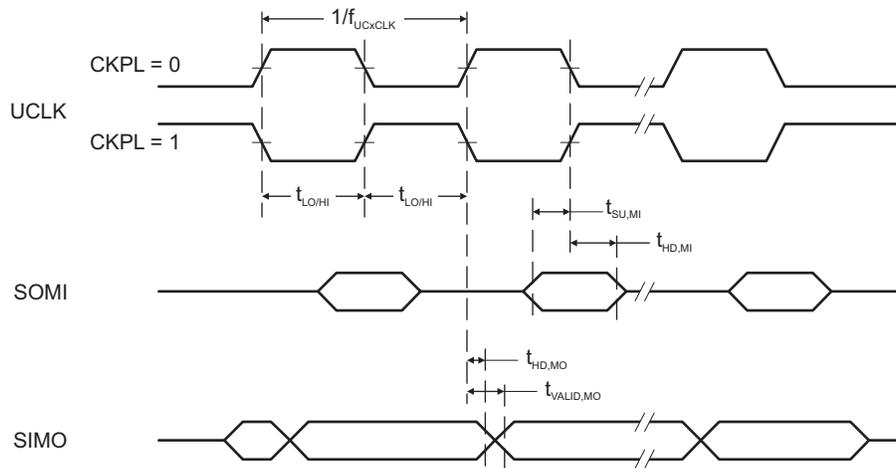
**Figure 5-16. SPI Master Mode, CKPH = 0**
