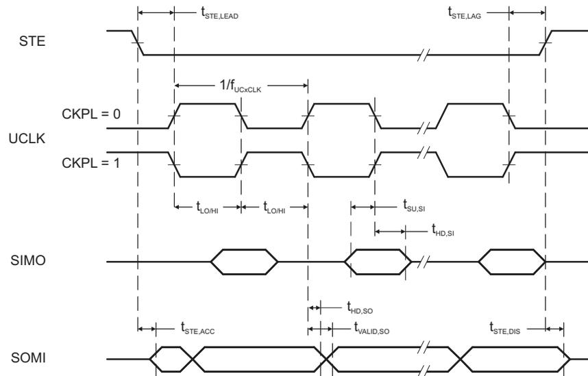
Figure 5-18. SPI Slave Mode, CKPH = 0
