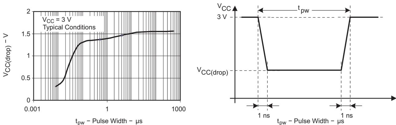
Figure 5-13. V<sub>CC(drop)</sub> Level With a Square Voltage Drop to Generate a POR or BOR Signal
