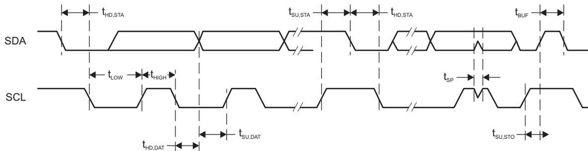
Figure 5-20. I<sup>2</sup>C Mode Timing
