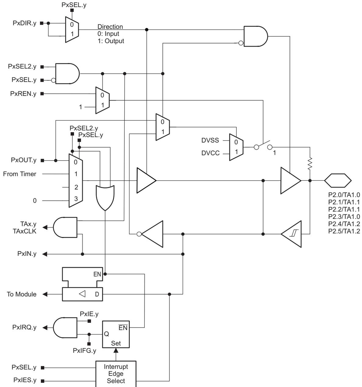
Figure 6-10. Port P2 (P2.0 to P2.5) Diagram
