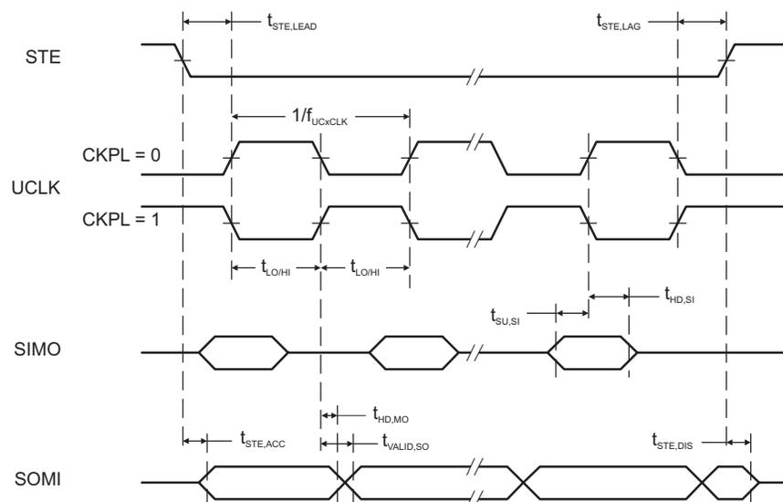
Figure 5-19. SPI Slave Mode, CKPH = 1
