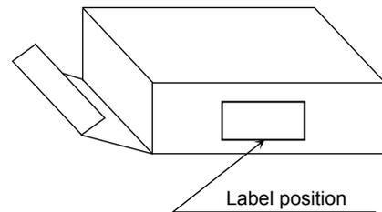
• The aluminum package in which the reel is supplied also has the label attached to center of one side.
