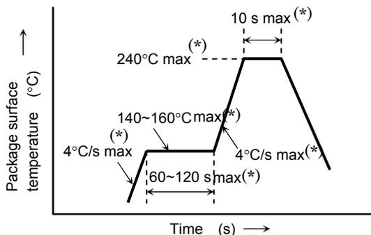
Temperature profile for Pb-free soldering (example)
