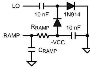
Figure 40.  $R_{RAMP}$  to  $-V_{CC}$  for  $V_{OUT} < 7.5V$
