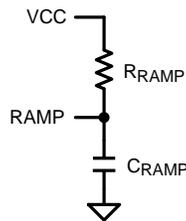
**Figure 39.  $R_{RAMP}$  to VCC for  $V_{OUT} > 7.5V$**
