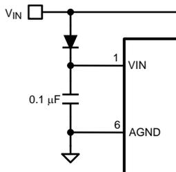
Figure 28. Input Blocking Diode for  $V_{CCX} > V_{IN}$
