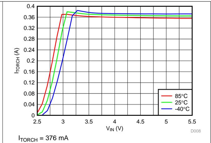
Figure 9. LED Torch Current vs Input Voltage
