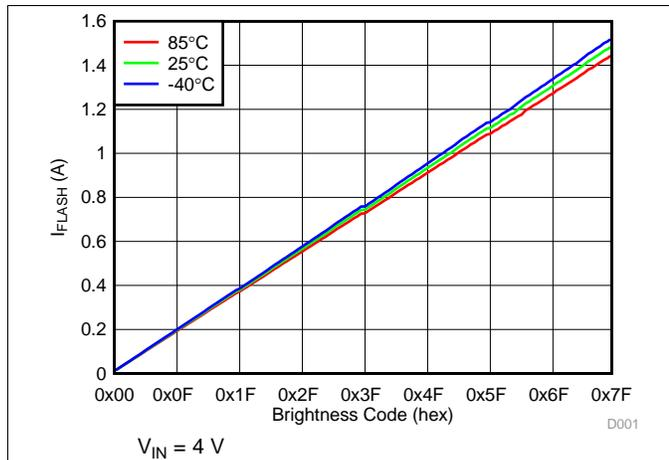
Figure 2. LED Flash Current vs Brightness Code
