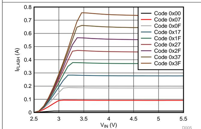
Figure 6. LED Flash Current vs Input Voltage
