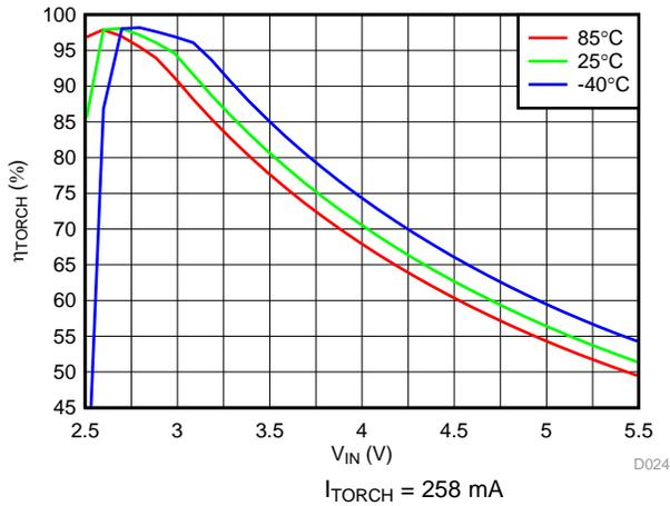
**Figure 33. LED Torch Efficiency vs Input Voltage**
