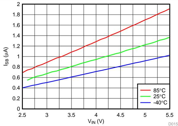
Figure 16. Standby Current vs Input Voltage
