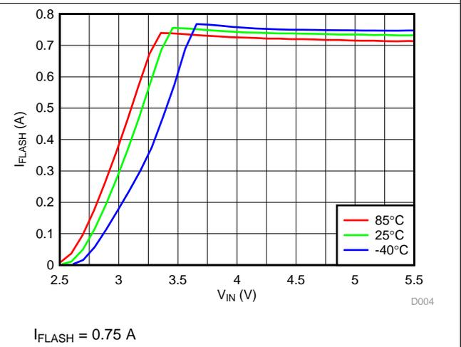
Figure 5. LED Flash Current vs Input Voltage
