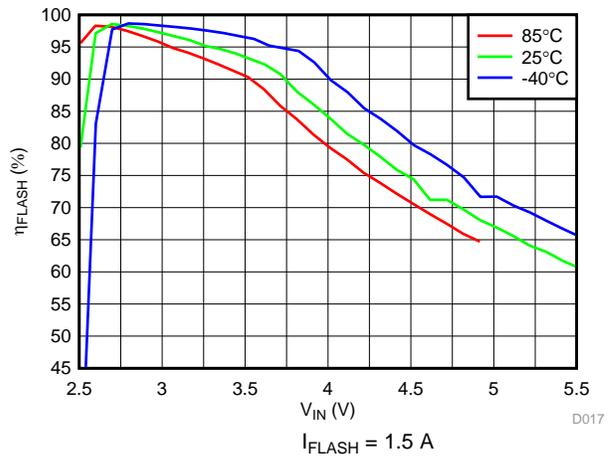
Figure 26. LED Flash Efficiency vs Input Voltage
