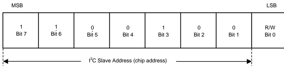
**Figure 23. I<sup>2</sup>C-Compatible Chip Address**
