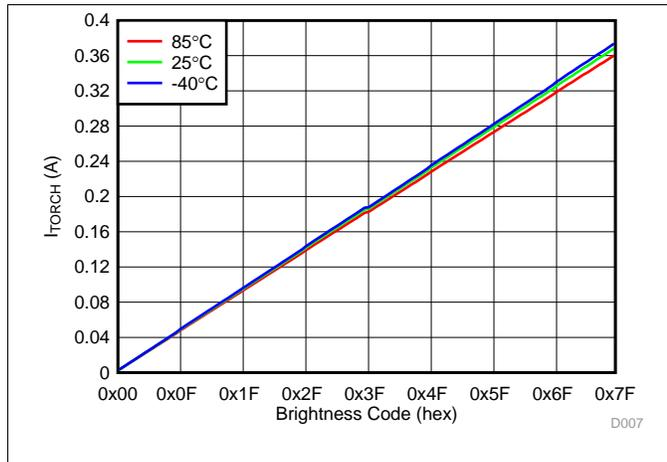
Figure 8. LED Torch Current vs Brightness Code
