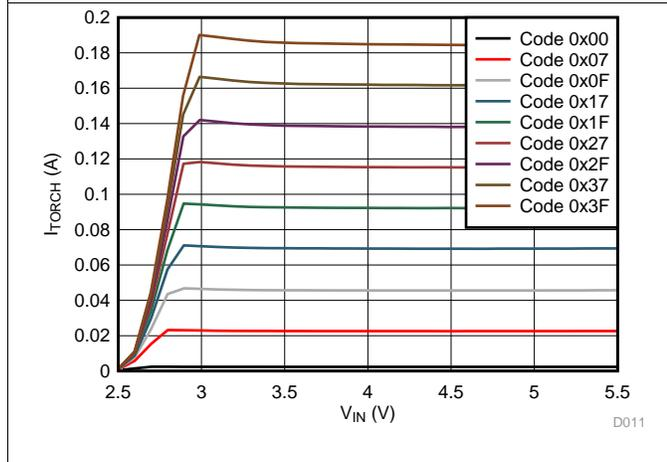
Figure 12. LED Torch Current vs Input Voltage
