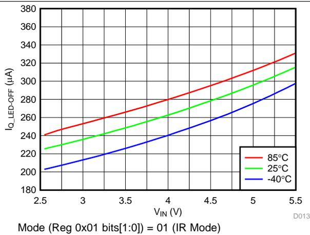
Figure 14. LED Off Current vs Input Voltage
