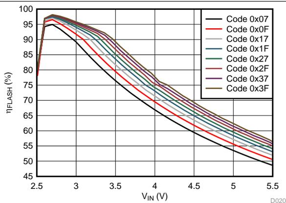
Figure 29. LED Flash Efficiency vs Input Voltage
