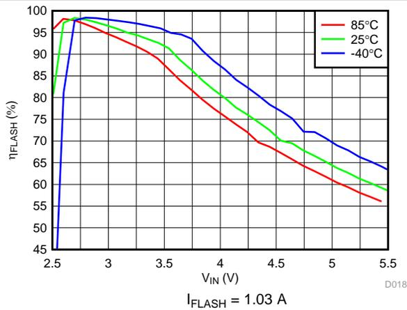
Figure 27. LED Flash Efficiency vs Input Voltage
