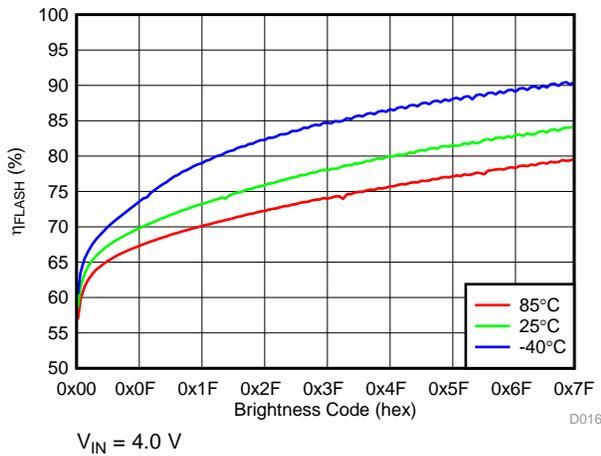
Figure 25. LED Flash Efficiency vs Brightness Code
