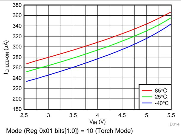
Figure 15. LED On Current vs Input Voltage
