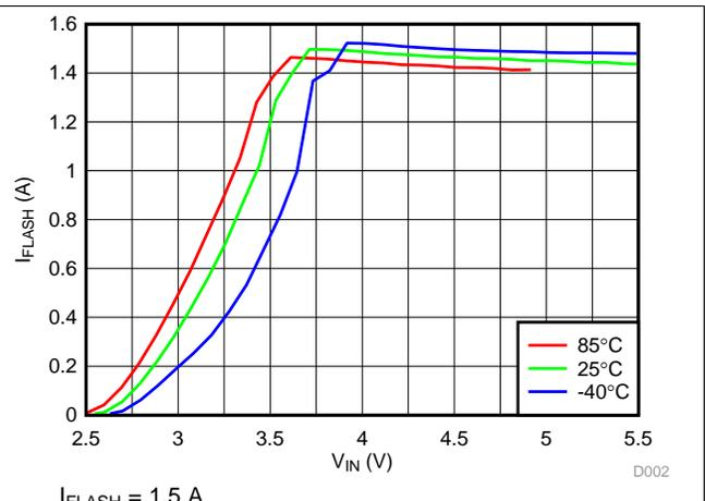
Figure 3. LED Flash Current vs Input Voltage
