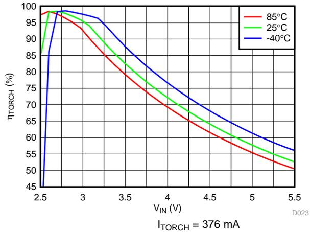
**Figure 32. LED Torch Efficiency vs Input Voltage**
