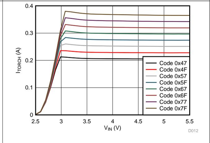
Figure 13. LED Torch Current vs Input Voltage
