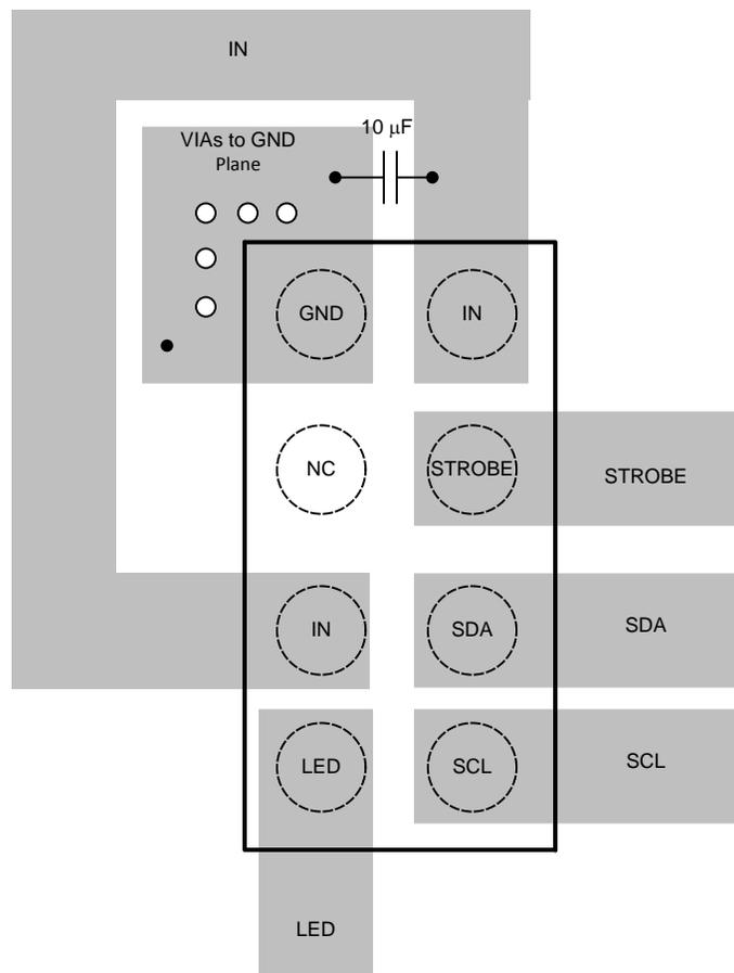
Figure 45. LM36011 Layout Example
