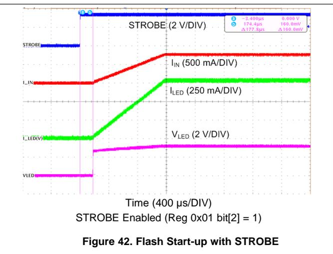
$T_A = 25^\circ\text{C}$ ,  $V_{IN} = 3.6\text{ V}$ ,  $C_{IN} = 10\ \mu\text{F}$ ,  $V_{LED} = 3.4\text{ V}$ , Flash Time-out = 320 ms and Thermal Scale-Back (TSB) disabled, unless otherwise noted.
