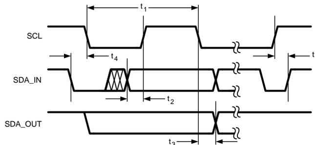
Figure 1. I<sup>2</sup>C-Compatible Interface Specifications
