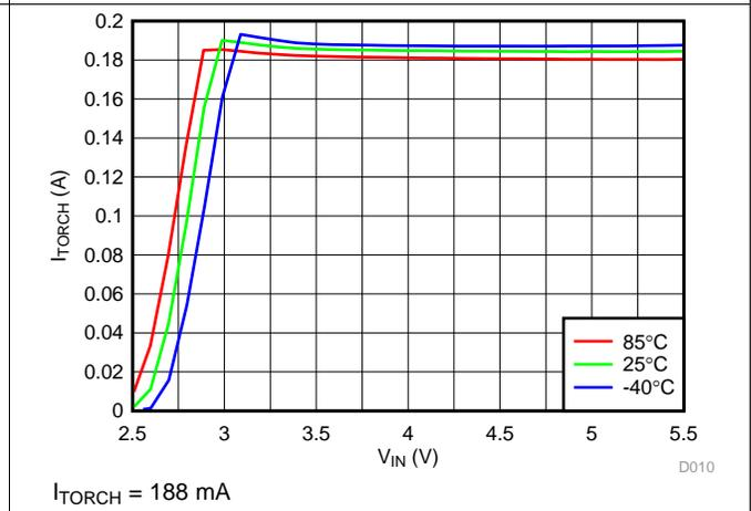
Figure 11. LED Torch Current vs Input Voltage
