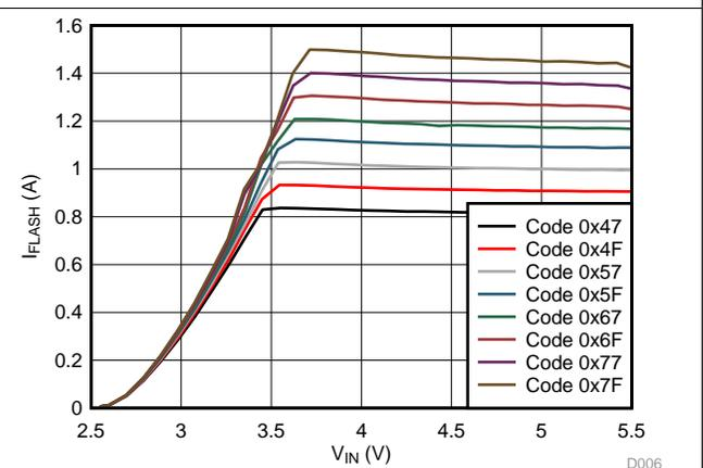
Figure 7. LED Flash Current vs Input Voltage
