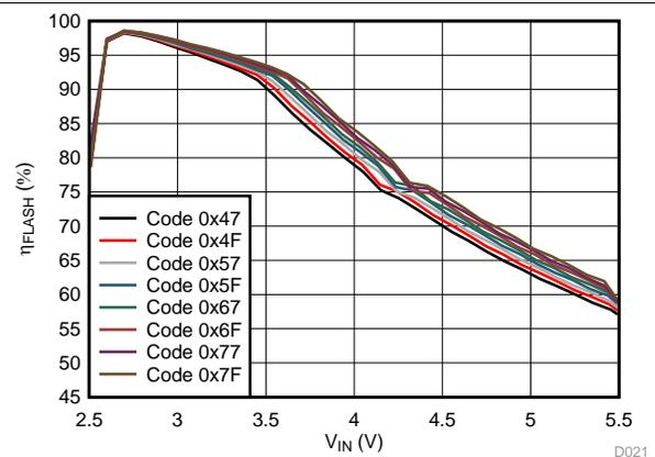
Figure 30. LED Flash Efficiency vs Input Voltage
