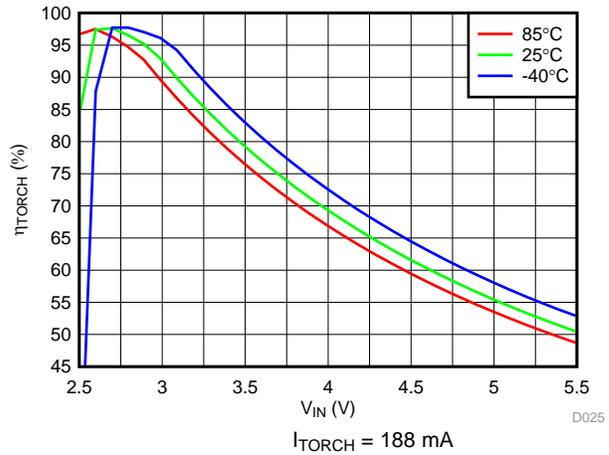
**Figure 34. LED Torch Efficiency vs Input Voltage**
