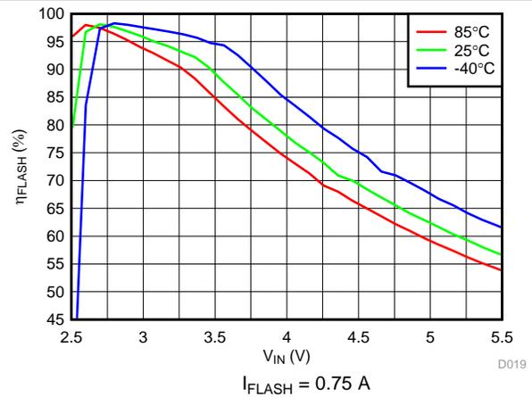
Figure 28. LED Flash Efficiency vs Input Voltage
