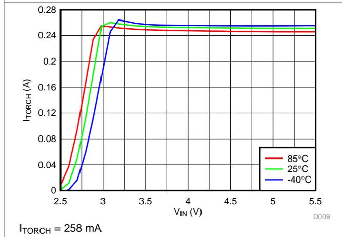
Figure 10. LED Torch Current vs Input Voltage
