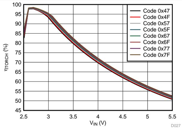
**Figure 36. LED Torch Efficiency vs Input Voltage**
