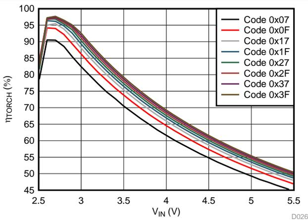
**Figure 35. LED Torch Efficiency vs Input Voltage**
