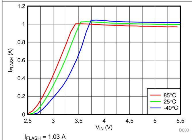
Figure 4. LED Flash Current vs Input Voltage
