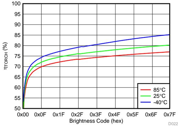
**Figure 31. LED Torch Efficiency vs Brightness Code**
