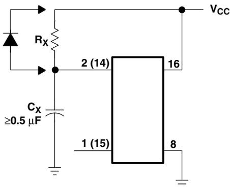
**Figure 5. Rapid-Power-Down Protection Circuit**
