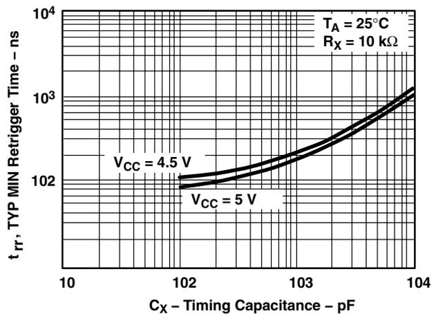
**Figure 4. Minimum Retrigger Time vs Timing Capacitance**
