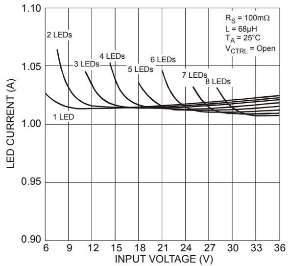
Figure 18 1A LED Current vs. Input Voltage
