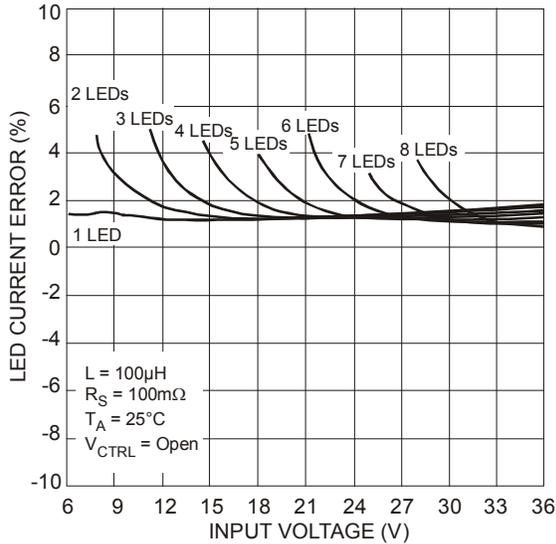
Figure 25 LED Current Deviation vs. Input Voltage
