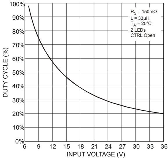
Figure 13 Duty Cycle vs. Input Voltage
