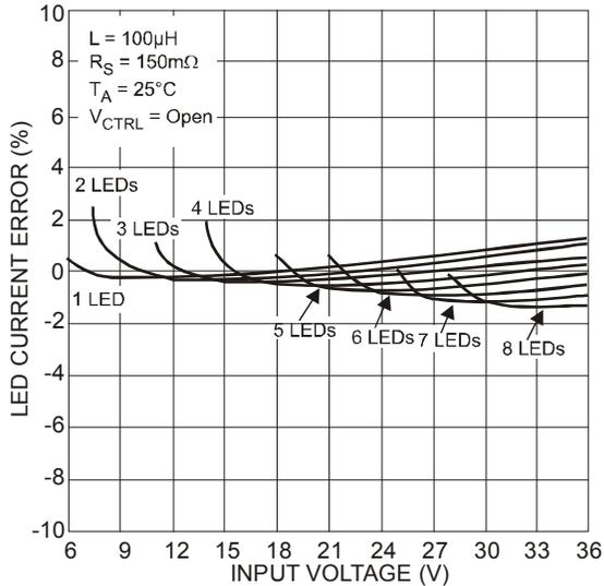
Figure 19 LED Current Deviation vs. Input Voltage
