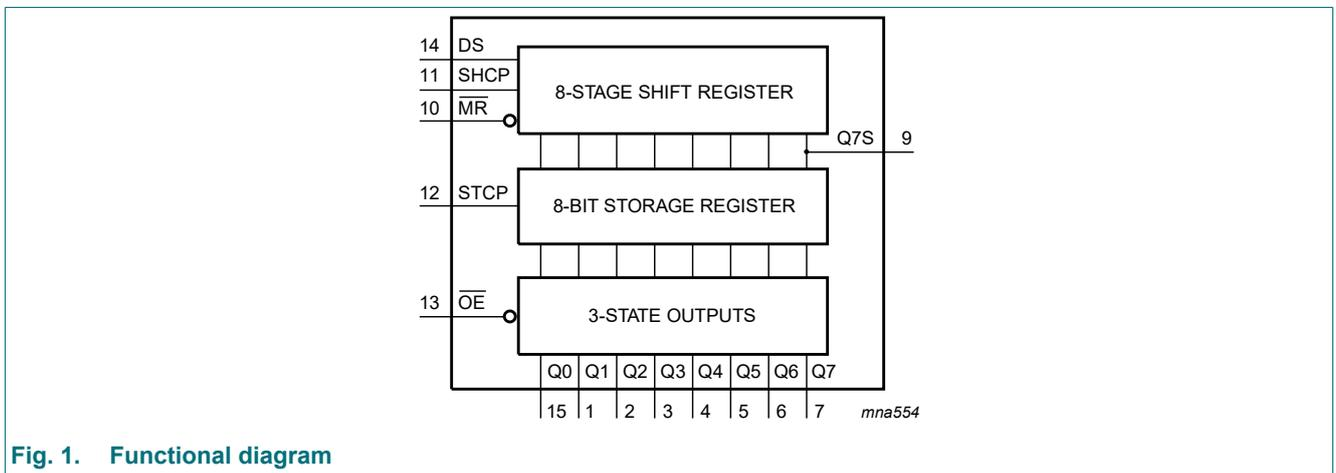
Fig. 1. Functional diagram
