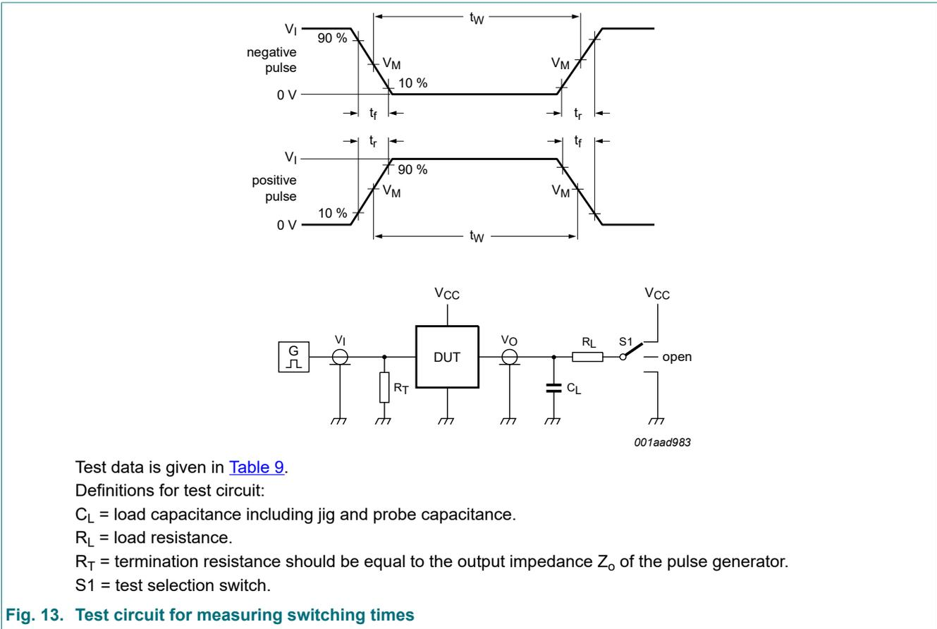
Fig. 13. Test circuit for measuring switching times
