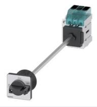
Load disconnector 3LD3, lu 32 A Main switch 3-pole Rated operating capacity for AC-23 A at 400V 11.5kW floor mounting Basic switch with door coupling Central hole mounting 22.5mm Toggle drive black 48x48 mm with auxiliary switch 1OE + 1S
