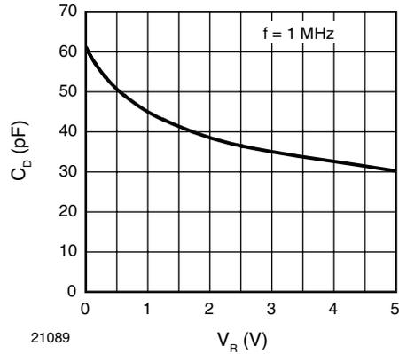
Fig. 6 - Typical Capacitance  $C_D$  vs. Reverse Voltage  $V_R$
