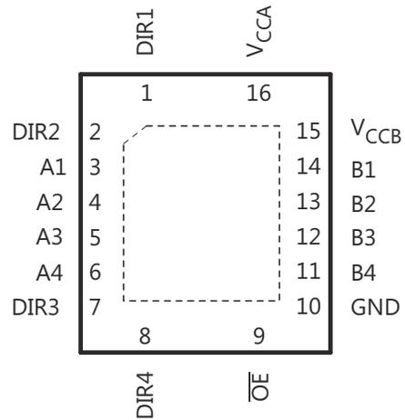
Figure 6-2. RGY Package 16-Pin VQFN Top View
