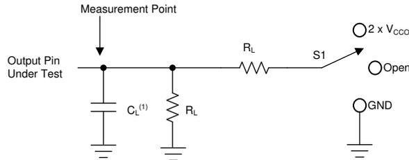
A.  $C_L$  includes probe and jig capacitance.
