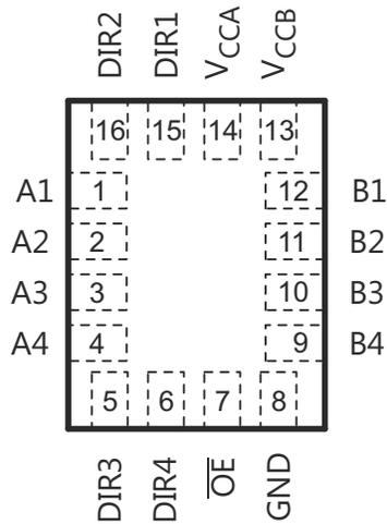
Figure 6-3. RSV Package 16-Pin UQFN Top View
