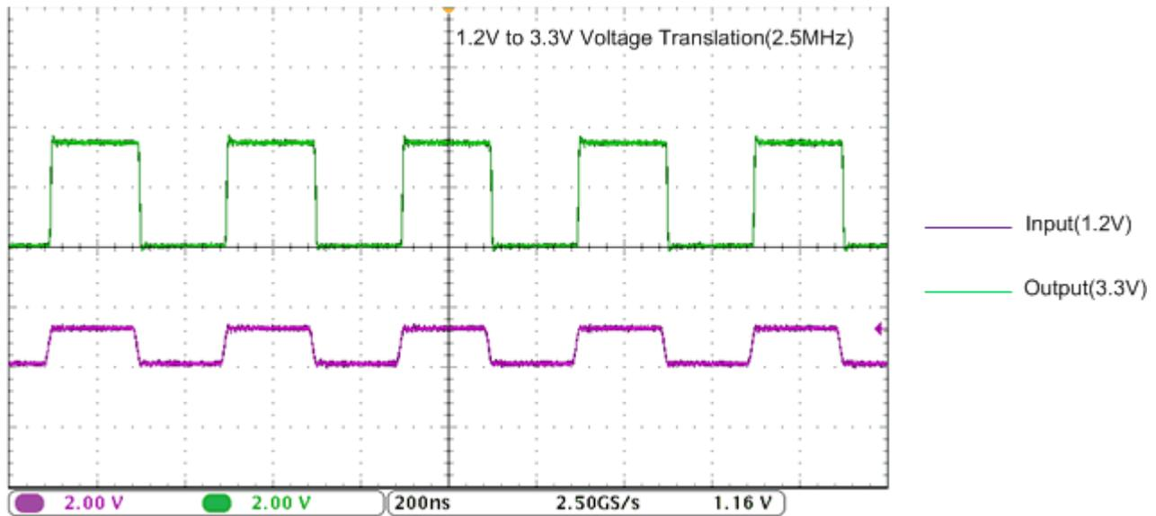
Figure 10-2. Translation Up (1.2 V to 3.3 V) at 2.5 MHz
