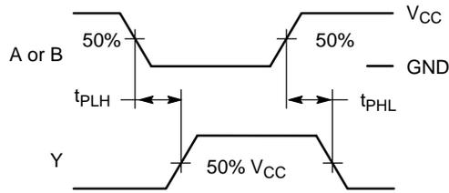
**Figure 3. Switching Waveform**
