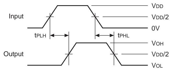
$$t_{sk(p)} = | t_{PLH} - t_{PHL} |$$
