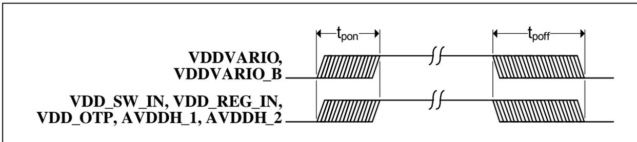
**FIGURE 7-3: POWER SEQUENCE TIMING (EXTERNAL REGULATORS)**
