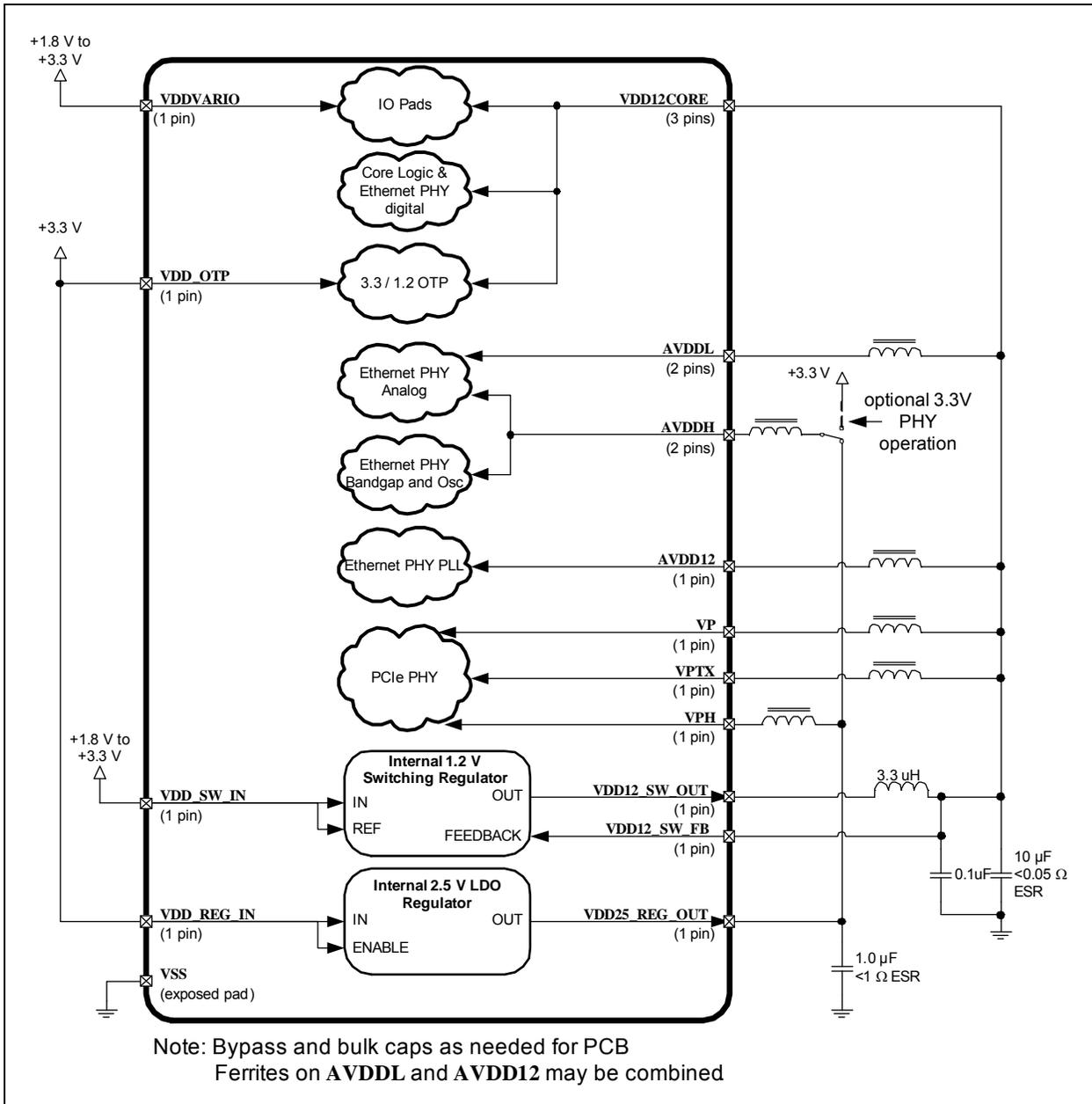
**FIGURE 4-2: LAN7430 POWER CONNECTIVITY ON-CHIP REGULATORS DISABLED**
