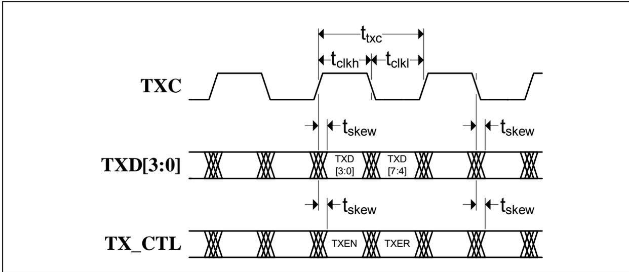
**TABLE 7-17: RGMII TRANSMIT TIMING VALUES (TXC INTERNAL DELAY DISABLED)**
