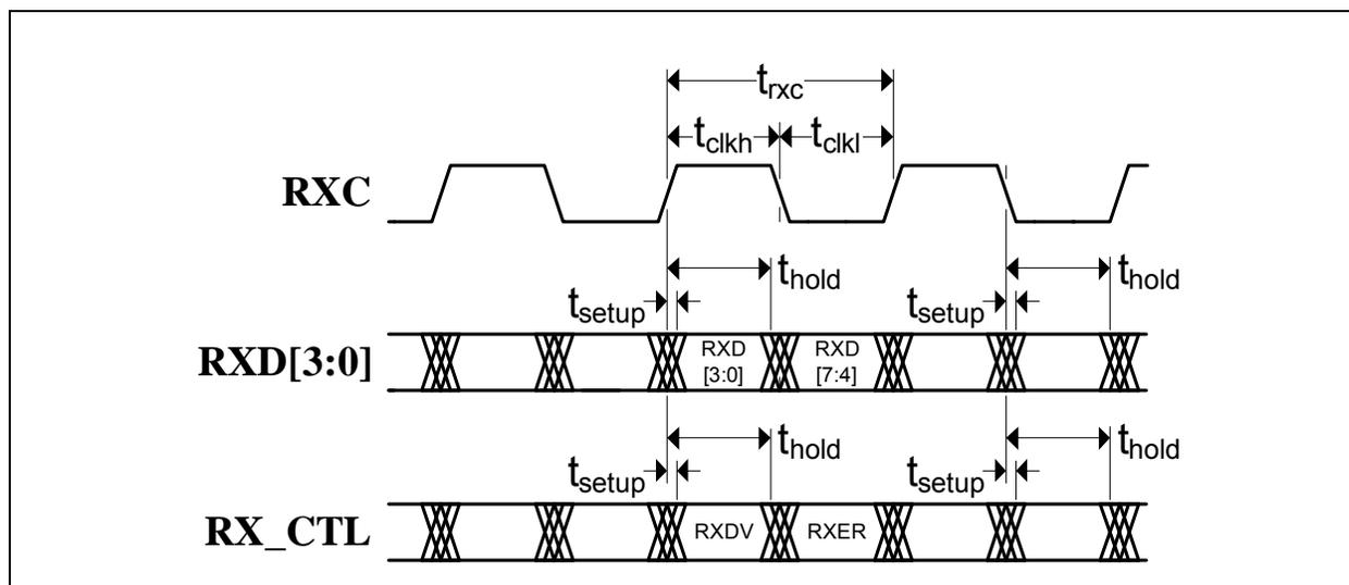
**TABLE 7-18: RGMII RECEIVE TIMING VALUES (RXC INTERNAL DELAY ENABLED)**
