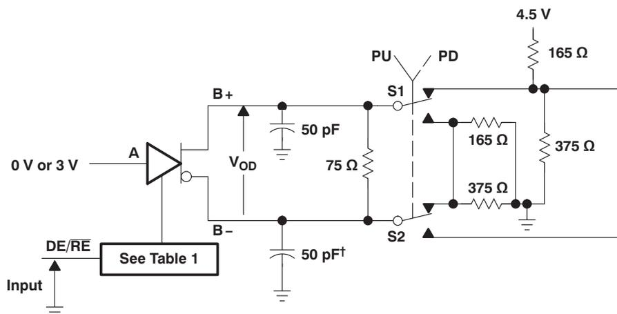
† Includes probe and jig capacitance in two places.
