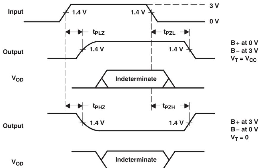
Figure 9. Receiver Enable and Disable Time Waveforms
