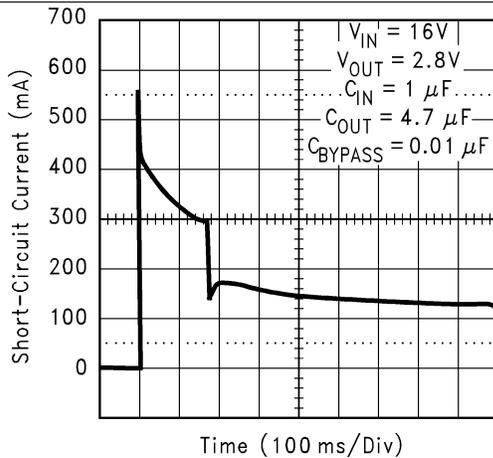
Figure 3. Short-Circuit Current
