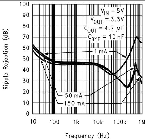
Figure 13. Ripple Rejection
