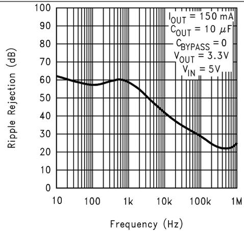
Figure 8. Ripple Rejection
