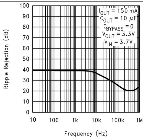
Figure 11. Ripple Rejection
