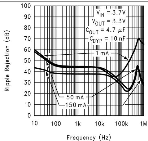
Figure 12. Ripple Rejection
