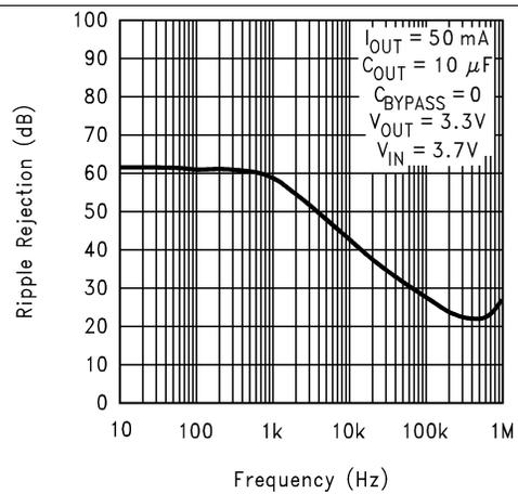
Figure 10. Ripple Rejection
