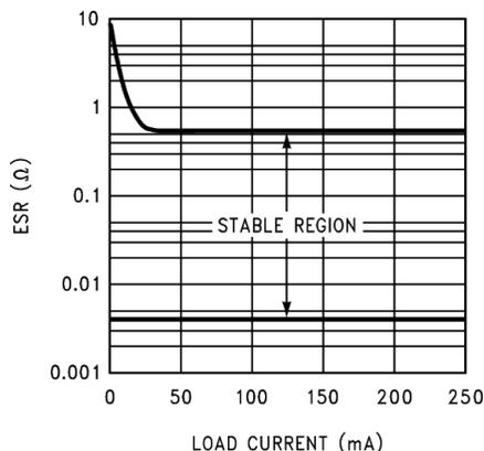
**Figure 35. Stable ESR Range vs Load Current**
