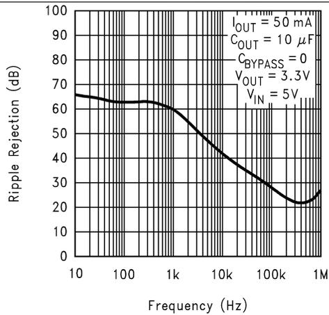
Figure 7. Ripple Rejection
