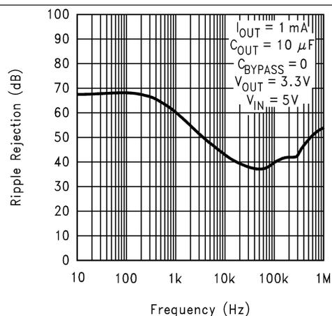
Figure 6. Ripple Rejection
