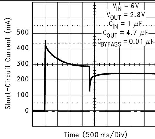
Figure 2. Short-Circuit Current
