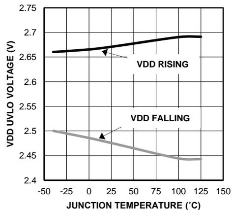
Figure 7. UVLO Thresholds
