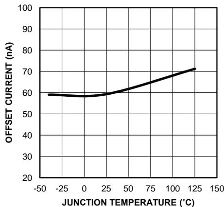
Figure 6. IDAC\_OUT Offset Current
