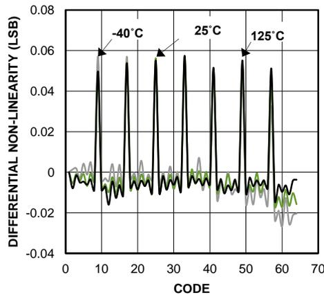
Figure 10. Differential Non-Linearity
