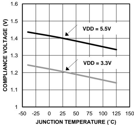
Figure 4. Output Compliance to Positive Rail
