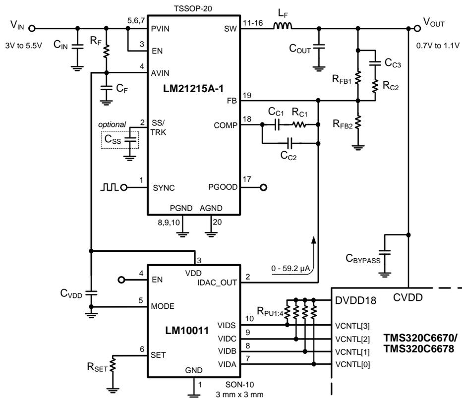
Figure 12. 6-Bit Mode Design Example
