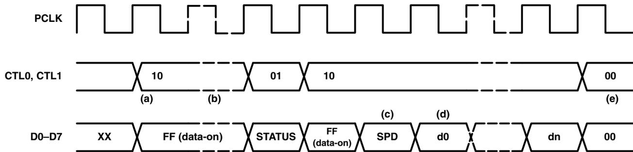
NOTE A: SPD = Speed code, see Table 35. d0–dn = Packet data. STATUS = status bits, see Table 32.
