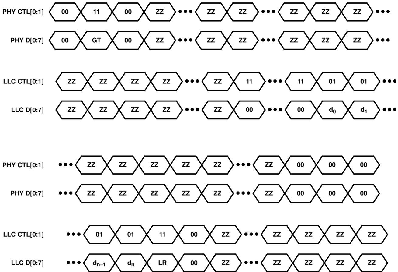
GT = Grant Type    LR = Link Request Type    d<sub>0</sub>–d<sub>n</sub> = packet data
