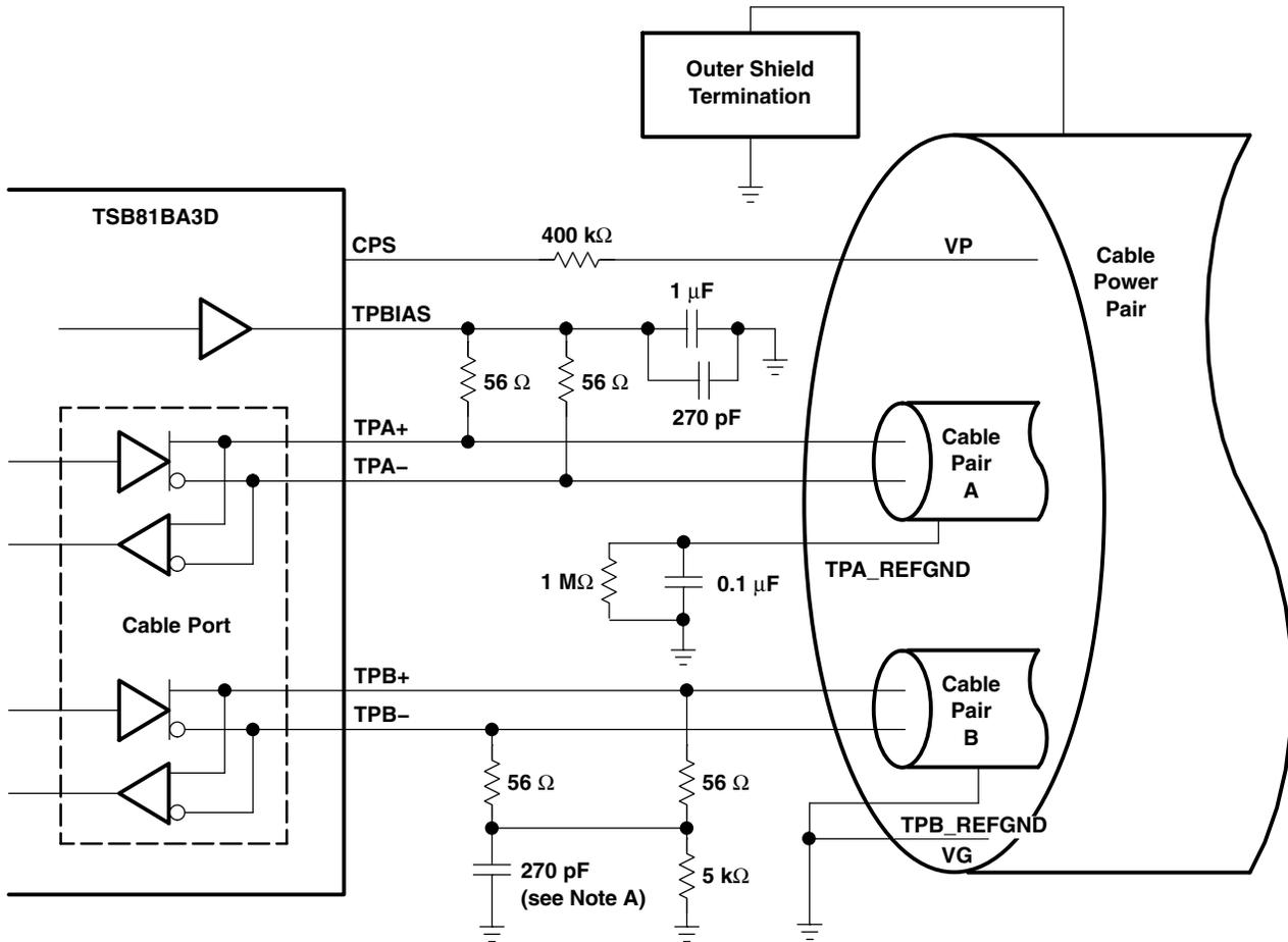
NOTE A: The IEEE Std 1394–1995 calls for a 250-pF capacitor, which is a nonstandard component value. A 270-pF capacitor is recommended.
