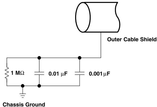
**Figure 5. Typical DC Isolated Outer Shield Termination**
