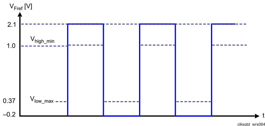
Figure 6-3. External Fast Clock (Square Wave, DC-Coupled)
