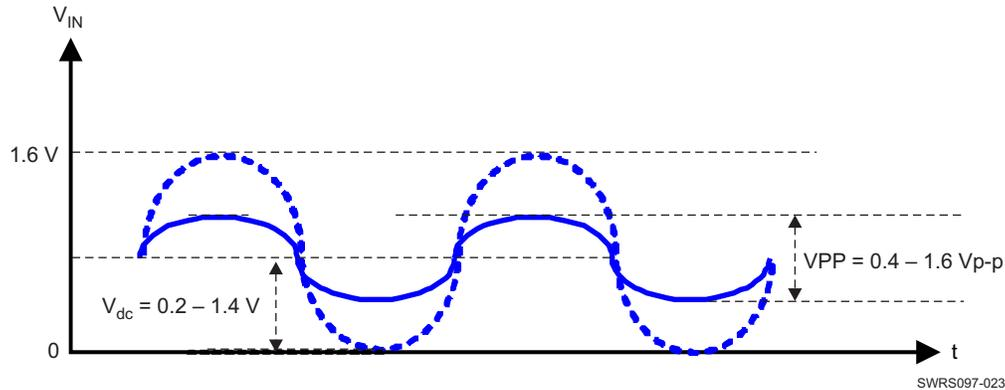
Figure 6-5. External Fast Clock (Sine Wave, DC-Coupled)
