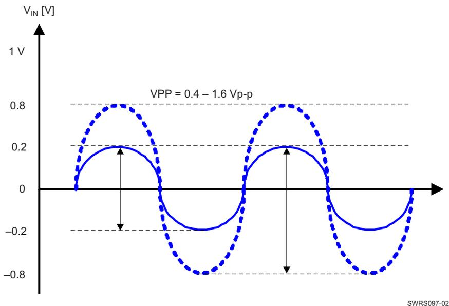
Figure 6-7. External Fast Clock (Sine Wave, AC-Coupled)
